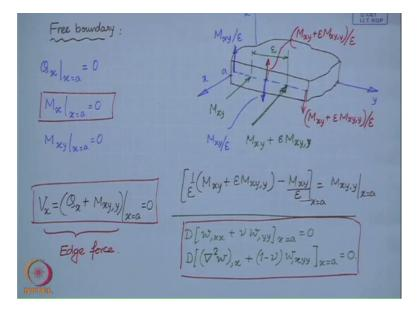
Let us discuss the free boundary. So if a plate has a free boundary then intuitively we may guess that so suppose this is X equal to A. So this boundary is at X equal to A. So intuitively we might guess that so this shear stress resultant so this QX is going to be 0 so QX is along z on this space so that should be 0. The moment = 0 and in addition we have another moment because of the shear stresses in-plane stresses that also has to be put to 0.
