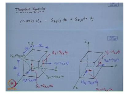
So these are the moment resultant now we can write down the equations of motion. (Refer Slide Time: 31:00)
