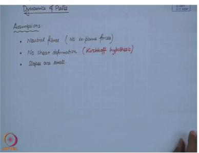
So the first thing that we assume that there is a plane or there are fibers which are unstressed these are called neutral fibers. So we assume the presence of neutral fibers which occurs if you do not have in-plane forces in the plate. So the plate is not subjected to any in-plane forces then you have when the plate undergoes transverse small transverse vibrations then there are fibers which remain unstrained.
