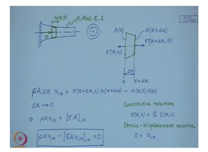
So with these 4 assumptions, we are going to now look into the equation of motion of a bar in axial vibration. So let me draw a bar, so this bar is made of material of density, say rho as an area of cross section A; which may be a function of the spatial coordinate x, has young's modulus E and has the length 1. Now at any location x of the bar, the displacement of cross section in the axial direction is measured by this field variable u, as a function of x and time t.
