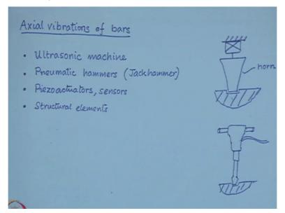
So today we are going to look at 2 examples on vibrations of one dimensional elastic structures that we have started with strengths. So today we are going to look at axial vibrations of bars and torsional vibrations of circular bars. So let us begin with axial vibrations of bars. So where do we finds bars in axial vibrations? So some examples are; in an ultrasonic machine, so in an ultrasonic machine, what you have is a bar which is shape like this, which is connected to an actuator.
