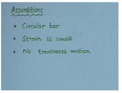
So once again for the mathematical model of such a bar, you make some assumptions, so the first assumptions that we make is that the; we have already said that the bar is circular, so we are going to study only torsional vibrations of circular bars that is to ensure that there is no wrapping of the cross section. We will assume that the strains are small, so that the dynamics can be adequately described by a linear model.
