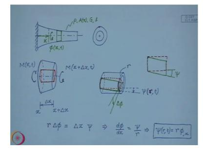
And we will also assume that there is no transverse motion. There is no transverse motion of the bar. So with these assumptions, let us look at a circular bar, so here I have a circular bar, made of material of density say rho as an area of cross section, which may be a function of the special coordinate x, the shear modulus or the modulus of rigidity is represented by G and this has a length l.
