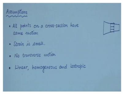
Now in order to model the dynamics of bars in axial vibrations, we begin with some assumptions that we make on this modelling. So the first assumption that we make is that all points of the bar are in all points on a cross section, have same motion. So what I mean by this is suppose you have a bar, at a certain cross section all points will have the same motion. The second assumption is that we make is that the strains, the strain is small.
