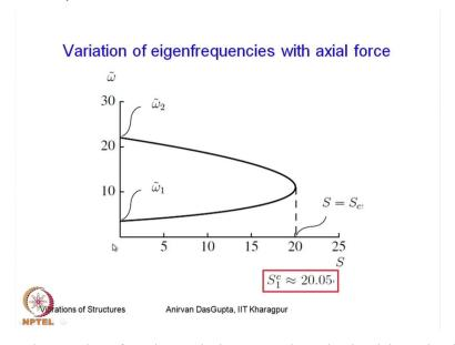
So here this shows the results of such a solutions so when the load is 0 the first two circular natural frequency non-dimensional are these two points and as the load is increased as you can see that omega 2 decreases while omega 1 increases and they collies at the certain value of load, now this is the value which is critical because after this they vanish, now to see what happens to these - these Eigen circular Eigenfrequencies.
