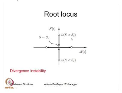
Now let us look at this picture in the root locus diagram, so s is the coefficient of the - in the exponential term in the solution so here I have plotted the real part of s and the imaginary part of s, so s is plus or minus I omega, so plus I omega tilde this is the minus I omega tilde, when the load is less than the critical load or the buckling load, as you increase the load these roots they go to 0, once they reach 0 then they move on the on this axis.
