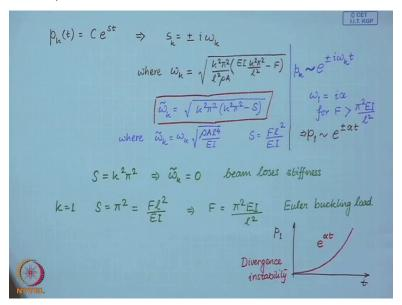
Now suppose we look for solutions of the form C times exponential s t, so if you substitute in here so, we will obtain solutions of s in terms of this omega k, where omega k is given by this expression, now we can make a little bit of simplification here by some redefinition we can write this, where so using this redefinitions we can recast this in - in this non-dimensional form the Eigenfrequency in the non-dimensional form.
