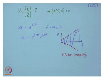
Now, so they can be recast as a matrix A times this is 0, so for non-trivial solutions of this coefficients the determinant of A and remember this A that A is the function of omega tilde and S the loading is must vanishing, so if you so you can solve for a given load S you can solve for the circular natural frequencies of the beam and this can be solved numerically.
