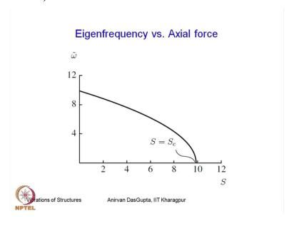
So here I have plotted this non-dimensional frequency circular frequency with the non-dimensional load so when the load is 0 you have this is the first circular natural frequency non-dimensional and as the load increases this falls and here at a certain load it goes to 0, the circular natural frequency goes to 0, so this is the buckling load and the critical load.
