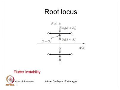
We look at the root locus which again we plot s the real part and the imaginary part of s, so remember that s is plus or minus I omega tilde, so when you have the - the load less than the follower force magnitude less than the critical value then these are the distributions of the circular natural frequencies plus or minus I omega 1 and plus and minus I omega 2, now as the load is increased these two come together and collies at a certain value which is the critical value of the load.
