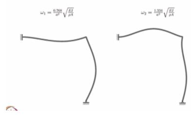
And we again perform the model analysis for this discretised system and if you do that then the result for the first 2 modes, so these are the first 2 circular Eigen frequencies of the system which has been calculated using this Lagrangian and expansion that I discussed just now. So this figure shows the first 2 modes of vibration of this plain frame, so you can see that, so this is the fundamental frequency and the corresponding Eigen mode of vibration.
