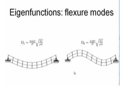
Now if you perform the model analysis of this discretised equations, then the first non dimensionalised circular Eigen frequency is obtained as 0.612, second one is obtained as 2.087 and so on. The fifth is obtained as 9.889, the sixth is obtained as, now there is a reason why I am writing 1,2 and then 5, 6, there are of course other circular Eigen frequencies in this range but let us look at the Eigen functions, which are shown here.
