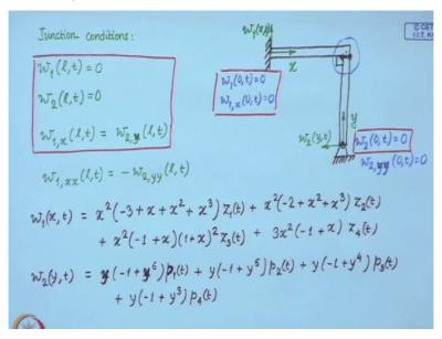
Now let us go over to a second example, this example is of a plain frame, so let us look at this plain frame. So we have this plain frame constructed out of 2 beams, which are welded at this point, so for simplicity, we consider that the lengths of both these beams is the same, so we have 1 and 1. Now here we have built in end of this frame and here it is a pin, pin end. Now these are essentially 2 beams, which have a junction.
