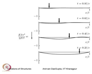
This figure shows the same thing when the speed is high. Now here you can see a difference from the previous figure, from the previous figure the deflection of the beam is completely on the negative side, below the equilibrium position. Now here at certain time instance, the beam goes above this equilibrium line.
