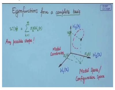
So what we mean by this? Suppose we have these Eigen functions, let us call them. Now there are infinitely many Eigen functions as we have seen. So here I can draw only three and with a little stretch of imagination, you can think of this as an infinite dimensional space with each axis labelled with one Eigen function. So any point in this infinite dimensional space with coordinates alpha 1, along W1, alpha 2 along W2, alpha 3 along W3, etc.
