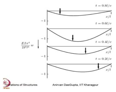
So this, this figure shows snapshots at certain time instance of a force travelling on a beam. So you can see how the beam deflects at various time instance. Now this is for the low speed. (Refer Slide Time: 42:19)
