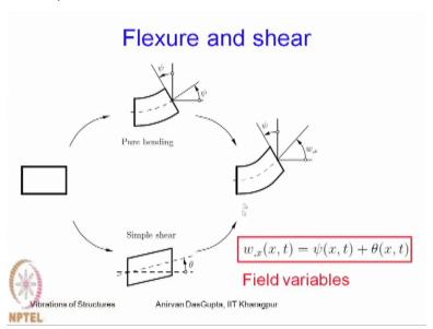
So the total picture looks like this, so this is the pure bending picture this is a simple shear picture and the net result is shown here now you can see that this shear because of this shear the
