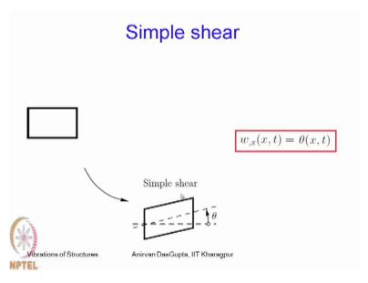
Now let us look at this case of Simple shear, when the element undergoes a simple shear so here this is - this simple shear is a - is a volume preserving deformation so this angle theta is the shear strain this is the angle that is the shear strain and as you can see here that the slope of the neutral fibers or the axis is nothing but this shear strain.
