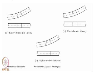
So in this figure I have shown this Euler Bernoulli theory, so what it says is that plane sections it will remain plane as well as perpendicular to the neutral plane neutral axis so this must be perpendicular here and still remains perpendicular, in the Timoshenko theory this was plane section still remains plane but now it need not be perpendicular to the neutral axis. Now you can then think of higher order theories in which plane section need not at all remain plane.
