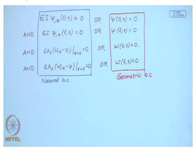
Now we have two field variables and corresponding to this two we have the for example for this, so this equal to 0 or psi so these are the connected by or these are conjugate so this is the angle and this is the bending moment and at 1 so these are the possible boundary conditions obtained from here and from here and similarly at x equal to 1, so these are the possible boundary conditions that we have that we can usually have there are other possibilities.
