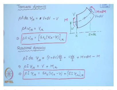
Now so we have these forces and moments let us look at the free body diagram of this beam element, so this is an exaggerated view so this is the transverse deflection at x at time t, here we also have this shear force and the bending moment, so if you write down the Transverse dynamics for this element.
