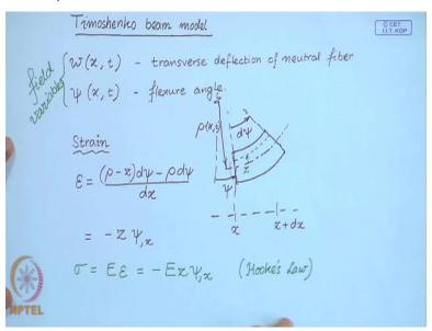
So this is the transverse deflection and this is the flexure angle, so these are the two field variables that we will use. Now let us then start representing our deformation in terms of these field variables. So the first thing is the strain so the fibers strain transverse to the in the - in the longitudinal direction of the beam. So if you once again consider fibers at height z from the neutral plane or the neutral axis.
