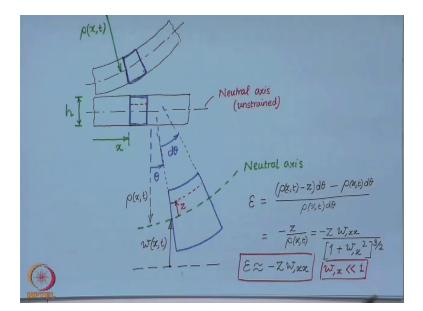
So once again let me draw this section of the beam, so this is our neutral axis or neutral fiber now this is neutral which means it is unstrained it reminds unstrained so this access in the undeform configuration and in the deform configuration it remains unstrained, so once again let us consider this element which upon deformation. So this is an element which undergoes deformation let the depth of this beam or height of the beam be denoted by h.
