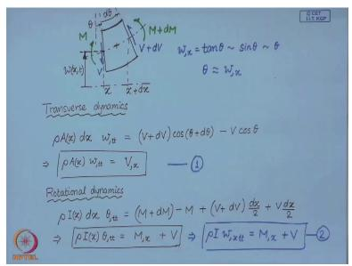
So now let us once again look at the free body diagram of this little element of the beam and introduce the interaction forces, so we have the shear forces at these faces and the bending moments so the sign convention what we follow so this is the positive shear force and bending moment and this so this is the undeformed neutral axis so this deflection is w x, t.
