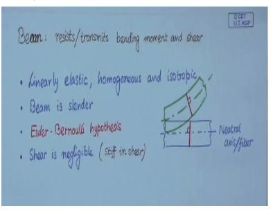
So a beam can resist or transmit bending moment and shear and it is a one dimensional elastic continuum, so this is a distinctly different from the definition of a - of a string which cannot
