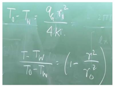
Here, this is the temperature scale, this is Tw and this is T, T as a function of r, so that means it is a parabolic distribution symmetry about r is equal to 0, very simple. You can find out dQ/dr at the surface.
