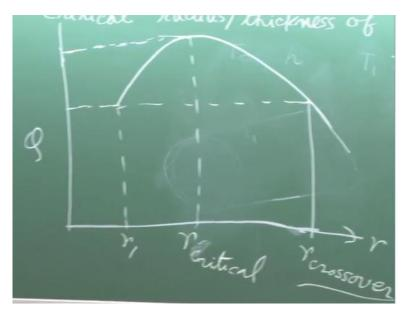
Then immediately we can make a draw a figure like this at r2 is K by h, it has a maximum. That means if I now draw a figure, that heat transfer rate Q verses r2, sorry, it has a, then it decreases. This is r1, this is this value K by h and this is known as r critical, or sometimes rc is equal to K by h. So, this is r critical, this is r critical. This axis is r2 rather r you can tell, r critical.
