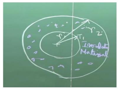
Now if you do so, let us draw this here again, front view that is r theta plane, let us have this insulation. I am only drawing the outer surface. The problem is forced with outer surface at T1. And now you put insulating, this is insulating material, this will look good, this is insulating material. And let us describe this radius r1 and let us consider the insulation is given up to a radius r2.
