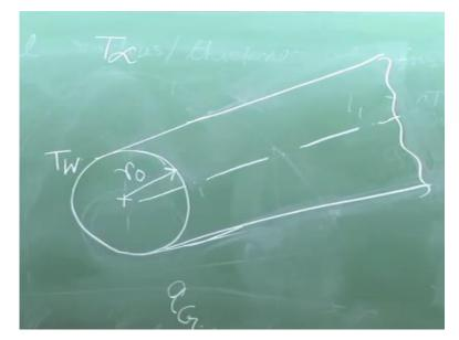
Let us consider a problem like this, we have a cylindrical rod, solid rod of radius r0, thermal energy is generated, which is specified by, the thermal energy generated per unit volume at a point, which may be a function of r. It is a one-dimension problem, so qG may be a function of r that is the radius of this solid cylinder, r may be constant. That means the volumetric heat generation rate is same at each and every point.
