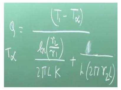
Now if you write the heat transfer equation Q, as you know that now this becomes a series problem as you have already done, from T1 it goes via conduction through the path, r2 minus r1. Then from here by convection to the surrounding T infinity with a heat transfer coefficient h. Now I can write the rate of heat transfer connecting the extreme potential that T1 by which the problem is prescribed.
