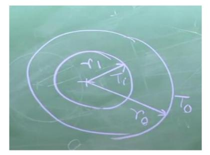
This is extremely simple problem. I do not know whether there can be any problem simpler than this, ri and r0 whose temperatures are maintained at Ti and To, o is outer, surface temperature. No ambience, nothing. You can see, can you this thing? Now cylinder conductivity, thermal conductivity is temperature dependent, so long in the class Prof. Som has talked about constant thermal conductivity.
