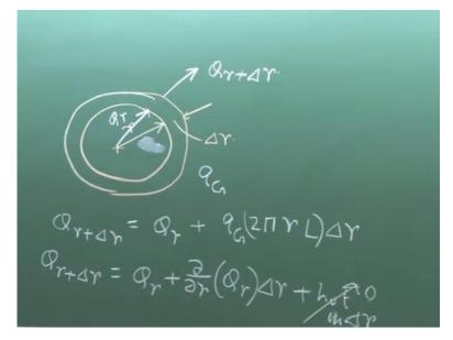
For clarity, I write here the annular ring. This is at an orbit value radius r, with this one delta r, then our same analysis what we do is that if Qr is the heat flux incident on this inner area, then this is the dimension, I am sorry. This Qr is the heat and heat going out is Qr plus delta r. The equation is very simple. If we consider a heat generation per unit volume qG within the cylindrical wall with extent from r1 to r2.
