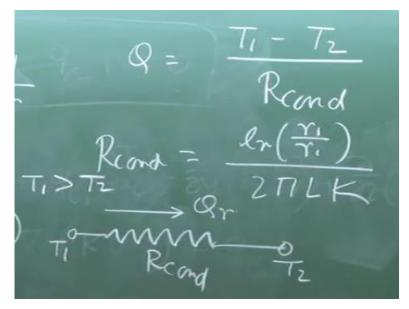
So, therefore if I write Q is equal to T1 minus T2 divided by conduction resistance. This conduction resistance is equal to ln r2 by r1 divided by twice pi LK, that means this can be represented by electrical analogous circuit like this, that this is the Qr radial direction, this is T1, this is T2, 2 potential T1 greater than T2, T1 greater than T2 and this is the R conduction, which is in case of plane surface it was L by K.
