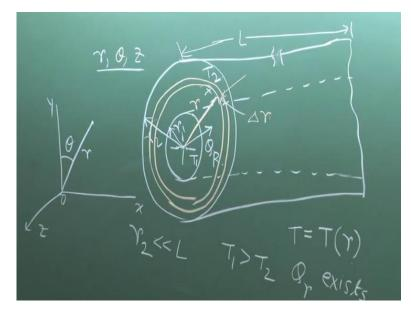
Let us consider a cylinder like this and the problem is specified like this, which we will be discussing. Let this be the center. The cylinder with inside radius r1 is cylindrical tube, outside radius r2, that means this portion is the solid cylindrical wall type of thing and the length of this cylinder is L and the problem is like this, r2 the outside radius of the tube, outer radius is very less than L, that means length is much more than the radius.
