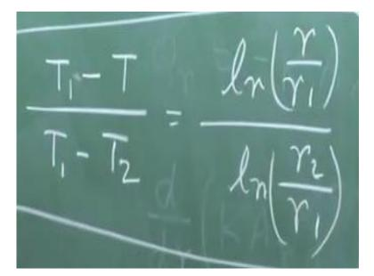
If you use these two boundary conditions, you get a profile temperature distribution T1 minus T divided by T1 minus T2. T1 is the inner surface temperature, which is higher than T2 is equal to ln r by r1 divided by ln r2 by r1. It is very simple that you substitute this to find out T1 and T2. T is equal to T1 ln r1 plus C2 and T2 is T1 ln r2 plus C2 and you can find out T1, T2 and finally you get this as the logarithmic distribution.
