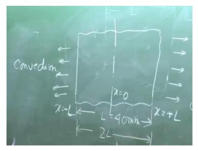
Instead, what is given the temperature within the solid is A plus Bx plus Cx square where A is 82.0 degree Celsius, B is minus 210 degree Celsius per meter and C is minus 2 into the 10 to the power 4 degree Celsius per meter square, x is in meter. Origin of the x coordinate is the meet point that I have already shown.
