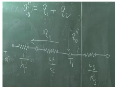
Without writing the equation, if you understand this, then it will be better that now the radiant heat, this is the node at bonded surface, that is T1 and this is the T infinity, so this is q1, which suffers that Lf/Kf as resistance, a I am not writing because we are finding out the heat flux q/a, so therefore air resistance is this, okay and this resistance is 1/hf and here this resistance is Ls/Ks, so this is the electrical network.
