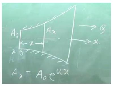
There is a rod like this the same thing which we did an application that I told the lateral surfaces are insulated. Now, x, this is x = 0 and the area is A0. Heat is flowing this direction because of the difference of temperature is mid, constant temperature at this phase and some constant temperature at this phase, temperature at this phase is more than this phase, which is not prescribed in the problem.
