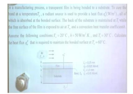
Now, this is a problem try to appreciate. I hope all of you can see. That problem requires a description. Well, in a manufacturing process, a transparent film is being bonded to a substrate. This is a statement of a practical process. This is a transparent film, which has to be bonded on a substrate.
