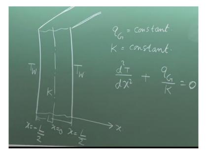
Now if you take the axis at the middle because of the symmetry of the problem, then boundary conditions are that at x=L/2, T=Tw, at the same time at x=-L/2, T=Tw. Now if we use this two-boundary condition, mathematically c1 will be 0, but this c1, 0 is obvious without writing the boundary condition, this is because the problem is symmetry, so that they are cannot be in any term containing x.
