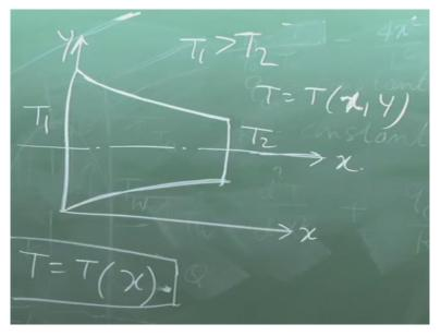
But we cannot neglect the variation of area, so therefore we cannot write the equation d square, dT, x square 0, because we know the general equation in these form, KA(dT/dx) +qG\*A=0. This is the basic equation, where from does it come? Your general heat conduction equation is not there A, coming into these, because there we have consider plane area.
