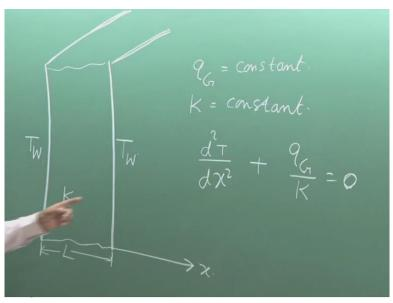
We discuss the analogous electrical circuit specifying the conduction and convection resistance. Today, we will discuss a simple classical problem of conduction, 1-dimensional steady state conduction heat transfer with heat generation. It is a simple but classical problem. The problem description is like this; again, a plane wall whose width is L, while dimension in the other directions; that means this direction perpendicular to the plane of the boat.
