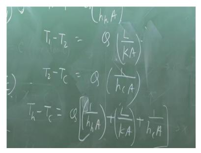
That means we can write this as Q is equal to Th - Tc divided by 1 by hhA + L by KA + 1 by hcA. That means this T1, T2 are eliminated that means if the problem is specified by the hot fluid in one side and cold fluid in one side and the heat is transferred from the hot fluid to cold fluid via the conduction due to the thickness of the wall then I can find out the heat flux knowing only hot fluid temperature and cold fluid temperature provided.
