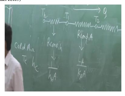
The same heat is going to that at this point there is heat continuity so this will be R conduction B. So, on has to understand these and if you can draw these thing KBA and this is R convection cold and that is 1 by hcA. So, if one can draw this electrical analogous circuit is a combination of resistances then probably may solve and we can write then Q as overall temperature difference if the problem is prescribed in terms of the overall temperature difference.
