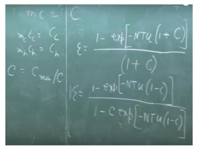
That means the capacity rate or simply the capacity and m dot c m dot c C c is the C c and m dot h c h is equal to C h and if I define C as the ratio of C min/c which may be either this by this that means this by this or this by this depending upon the case. In that case the expression will be
