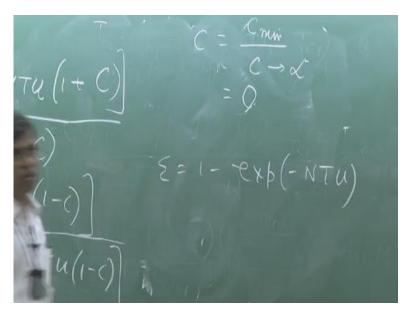
This higher C tends to infinity because which tends to infinity that will always be higher no question of calculation. That means an intelligent boy will tell that for boiling condensation the ratio which you denote as C will be always zero and if you put C zero in both the expression will yield the same value Epsilon is one minus exponential minus NTU this is the argument. If you put C zero because the ration is always zero.
