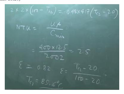
NTU is known, what is NTU? uA/C min. What is C? 2\*2=4 and this is 0.48\*4 that means which
