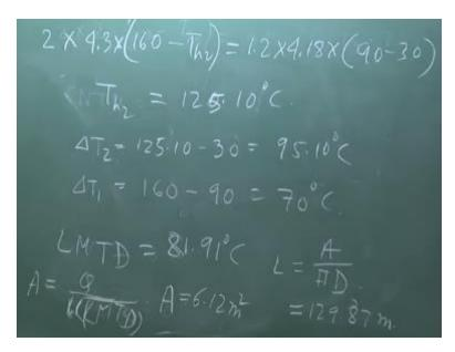
Water is 1.2 or the hot fluid first, hot fluid is; what is the flow rate? 2 into You tell me, you dictate me I will write, I will not see. First heat balance, 2\*4.3\*(160 - Th2) = 1.2\*4.18\*(90-30). What is the value of Th2? Nobody can tell without calculating it. Th2 is 120.10oC. Then Delta T2 125 -- sorry 125.10 - 130 is equal to 95.10 degree Celsius this is meaningless but still I am doing. Delta T1 is Th1 = 160 - Tc2 that is 90 that is equal to 70 degrees Celsius.
