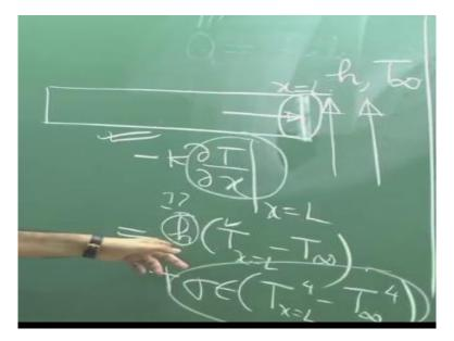
Let us say that the convective heat transfer coefficient is h, and the temperature is T infinity; ambient temperature is T infinity. So, h is the convective heat transfer coefficient and the ambient temperature is T infinity. So, what is the boundary condition here? The boundary condition here is that whatever heat flux reaches here by conduction, thus the same heat flux gets left from here by convection.
