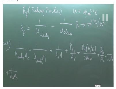
And that is expressed by a fouling factor denoted by R comes from the resistance this fouling factor expressed in terms of a resistance R and which his defined as—and because of that what happens thermal resistance enhances therefore the overall heat transfer coefficient gets reduced. Because thermal resistance is 1/u tens a reference area and therefore it is the heat transfer terminology in the practice that define the u dirty.
