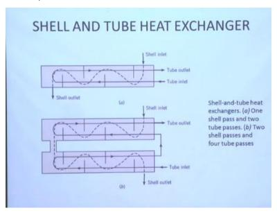
Now next I show you Shell-and-tube heat exchanger again for your practical information industry people will be very happy, this is what shell-and-tube type. Number one is one shell pass and two tube pass, that mean Tube inlet one direction again it comes out is a U tube type. Tube outlet that means in a U shape U comes here that means this is one pass and it comes likes that. That means inlet and outlet in the same side.
