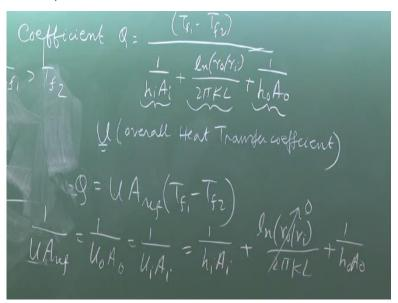
Then if you remember correctly than Q is equal to Tf1 – Tf2 that is overall temperature difference potential difference divided by 1 upon hiAi, if Ai is the inner surface area that means twice pie rl into L. I am not writing in this fashion, inner surface area plus if you remember ln(ro/ri) divided twice Pie kL plus 1 by hoAo which is twice pie ro into L that is outer surface area.
