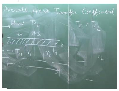
Let us consider this case again what we read earlier that there is a pipe I am drawing the symmetric part from the axis which has a fluid flowing through this pipe simply going back to the first few lectures, introductory lecture of heat transfer which I taught you. Fluid at a temperature of Tf1 and there is another fluid flowing through outside fluid which is at Tf2 that means the ambient fluid.
