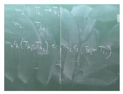
Now let us consider a situation like this, you have a duty fixed that means you have cool a hot fluid from Th1 to Th2 known. And you know that your cold fluid flow rate requirement available is this. And the cold fluid temperature available is this Tc1 which is usually the ambient temperature. So immediately a boy of class 8th will write mhch (Th1 – Th2) is equal to mcCc (Tc2 – Tc1) because entire heat exchange is insulated so from energy balance you will write and find out Tc2.
