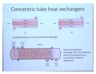
Now, I show you the most simple type heat exchanger is like this a concentric tube heat exchanger. This is the most simple-type we can conceive that there are a two concentric pipes one is the inner one and another is the outer one. So, one fluid flows through inner tube another fluid flows through the outer tube. Usually the hot fluid is flow-- allowed to flow through the inner one and the cold one is outer, but not necessarily.
