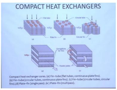
Now which is important little bit but still practical is Compact Heat Exchangers. This is very important. Employer asks, what is a compact heat exchanger? We want a heat exchanger which must have a very high heat transfer rate so that it mix the service require, huge service, we have to cool a hot fluid by a very high degree of cooling. That means the temperature difference is very large or the other way heating.
