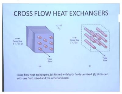
Now another type of cross flow heat exchangers is used, this before going to this I think well Compact heat exchanger, this also comes in the category of compact heat exchanger. First of all, I will explain this, this is another type of heat exchanger where the tubes side fluids are flowing through a number of tubes and where there are number of plates attach to these which acts as finned surface. Finned doing both fluids unmixed.
