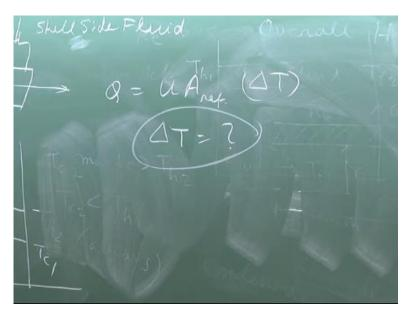
So, if I write this here for heat exchanger Q is equal to u -- let us take overall outer surface area uA or inner surface area, reference area A0 or Ai does not matter Delta T, what Delta T? This is a big question this Delta T changing. For example, in a parallel flow it is Th1 – Tc2 and not Th2 – Tc2, so Delta T is maximum at the inlet. In case of parallel flow this goes on decreasing which Delta T. Which I will take?
