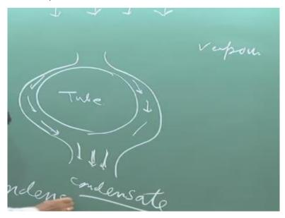
Just I tell you certain things that in the circular tube, usually what we use, it looks like that. If tube is horizontal like this a horizontal tube and if the vapour flows like this either push vapour or vapour flow, flow with a gentle velocity, then what happens it looks like this, the film grows; the picture is like this and tickles down the surface of the; this is the tube, tickles down the surface; this is the film, tickles down the surface of the tube.
