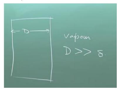
So therefore, different cross-sectional shape has been considered which keeps an effective gravity move, so that this can make the drainage of the condensate faster. Now in case of a vertical cylinder, the information is like this; in case of a vertical cylinder, condensation outer surface in the vertical cylinder, vapour is there. We can use the expression for vertical flat plate provided the diameter of the cylinder is much higher than the thickness of the liquid film, then we can use it.
