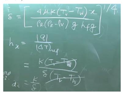
Therefore, I can write that delta is equal to 4 mu K Tv minus Tw x divided by rho l, rho l minus rho v g hfg, g is the acceleration due to gravity, hfg is the enthalpy of condensation whole to the power 1/4. This was Nusselt derivation for the growth of film, which is proportional to the fourth power of the x. If you compare it with the growth of boundary air over a flat plate in laminar flow.
