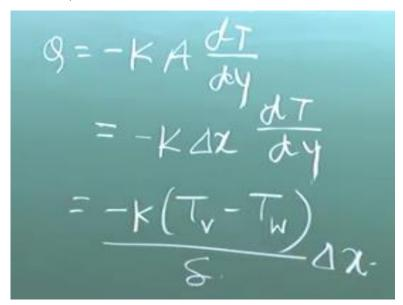
We have to find out what is Q. Q is equal to minus KA dT/dx, we know, here it is dT/dy. What is A for this control volume minus A into delta x, we have taken a unit v. What is del T/del y at this interface? Because here is a temperature Tv vapour site and here Tw it is less than Tv that means there will be some temperature gradient from Tv to Ty, which is decreasing in this direction of the plane. Well, now there is an assumption.
