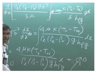
So, we get d/dx of rho l minus rho v into g delta Q divided by 3 mu is equal to, now we take the absolute value that is equal to K Tv minus Tw divided by delta. Now there is a delta, I am sorry, d/dx of m.x delta x is K tv minus Tw delta x divided by hfg, because Q by hfg. That means I am substituting this mass flow rate m.x from here and I am substituting the absolute value of Q here and I get this relationship, clear?
