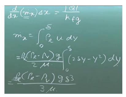
That means I can write d/dx of m dot x del x is equal to what I can write Q divided by hfg and here I deliberately put a mod value, absolute value of Q, because Q by hfg represent the rate of mass condense, which is a scalar quantity, so q may come out from some analysis with a positive and negative site, which will be so that q in the positive y direction or negative y direction of the problem.
