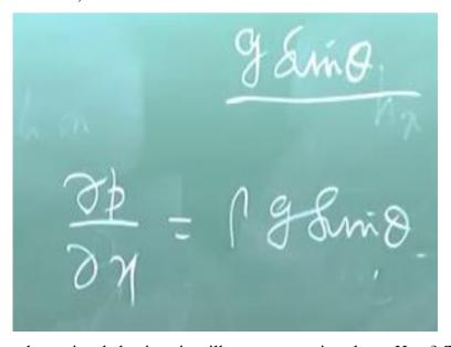
That means here the entire deduction, it will come as g sine theta. How? This is because obviously the effective g, which is working here is g sine. That means the weight, the component, the effective weight will be rho g sine theta along the direction of the flow and at the same time del  $p/del\ x$ . If this is x, will be rho g sine theta. So as a whole, a sine theta multiplication factor will come.
