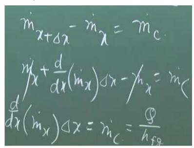
So, a simple mass balance of this control volume tell that m dot x plus delta x minus m dot x is equal to m dot c, simple. Primary school level thing that means the gross mass balance of this control volume is that m dot x plus del x is equal to m dot x plus m dot c and I am retaining that value and if I expand this in a Taylor series by neglecting the higher order term because of delta x is very small.
