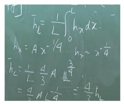
Now, if you are told to find out an average heat transfer coefficient over a length 1 of the plate, which is defined as this, 0 to 1. This is the definition of the average heat transfer coefficient over a flat surface, what is that value in terms of h1? Can you tell me? I told several times in the convection class. You have forgot, so I tell you again. Here, you see these things are all constant.
