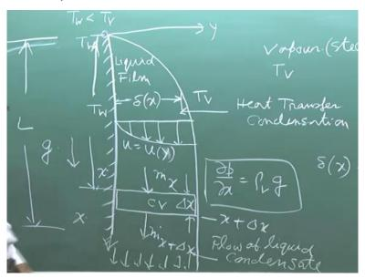
So, to understand film condensation let us consider this ways so that we can have a clear understanding. A simple case of a vertical flat plate, let us consider a vertical flat plate, which is at a temperature Tw and there is a vapour at saturated state, vapour at saturated state, whose temperature is Tv. Now this vapour you can consider as steam and if it is one ambient, one atmospheric pressure as the ambient pressure.
