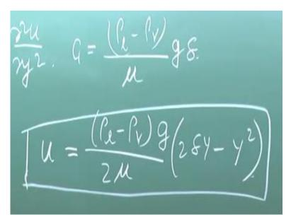
So, if you substitute this c1 here, then you get u is equal to rho 1 minus rho v, you take this rho 1 minus rho v by two mu g, then it will be two delta y minus y square. It is always positive, because rho 1 is greater than rho v and since y is less than delta, the quantity in the bracket is also positively proved that u is in the direction of the positive x axis, obviously, it is flow is dominated by the buoyancy, okay.
