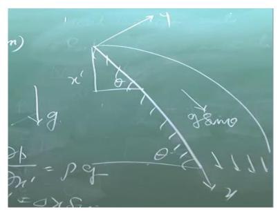
If the plate is inclined with an angle theta with the horizon, it is simply school level thing. So therefore, this is y and this is x, but g is in this direction. So entire thing will be changed by an effective g, g sine theta.
