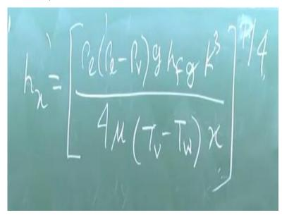
Then you get hx equals to K by delta. That means here I write hx is equal to this thing will go top, K by delta. That means K4 that means this will come, you just see rho l, rho l minus rho v into g hfg into KQ divided by this one will come 4 mu Tv minus Tw into x whole to the power 1/4. What happens K by delta, that means hx will be K by delta. This will be K inverse this and K4, I make and take it under one-fourth root, so it will be KQ, clear, Okay.
