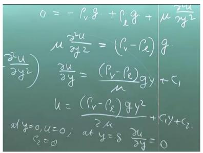
Now static pressure radiant in this vapour, vapour is stationary, so hydrostatic equation of pressure will hold good. So, del p/del x will be rho g, rho v, rho v is the density of the vapour, because we know del p/del x, it is because of the wet. This you know from your fluid mechanics knowledge the pressure filled in a hydrostatic. The pressure changes in the direction of the gravity.
