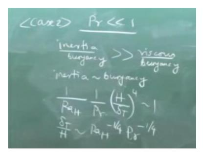
So, for Prandtl number much less than one, you have inertia by buoyancy is much greater than viscous by buoyancy, okay? So, inertia by buoyancy is much greater than viscous by buoyancy because the Prandtl number being less than one, one by Prandtl number will be much greater than one.
