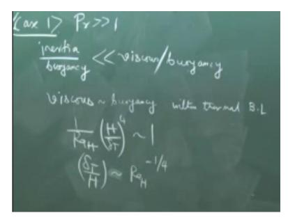
So, we will consider the first case when Prandtl number much greater than one. If Prandtl number is much greater than one then inertia by buoyancy is much less than viscous by buoyancy, right? Because other factors are the same. That means which forces are competing? Viscous and buoyancy within which boundary layer, thermal boundary layer.
