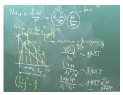
For Nusselt number is equal to hH by k which is equal to h delta T by k multiplied by H by delta T. This is of the order of one. We have shown that this of the order of one does not depend on whether its Prandtl number much greater than one or less than one and this is of the order of Rayleigh number to the power of one fourth to the Prandtl number to the power one fourth.
