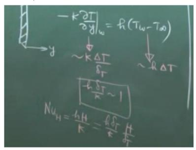
So, if this is the plate and this is the y axis, at the wall we can write minus k del T del y at wall is equal to H multiplied by T1 minus T infinity. Nusselt number is this H expressed in a non-dimensional form. So, what is the order of magnitude of this? Yes, what is the order of magnitude of this? K. The characteristic temperature gradient takes place within the thermal boundary layer.
