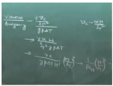
Viscous by buoyancy, viscous force nu vc by delta T square divided by g beta delta T. What was vc? Alpha H by delta T square, right? So, this is nu multiplied by alpha multiplied by H by delta T to the power 4 g beta delta T. So, this you can write it as g beta delta T, H cube by nu alpha multiplied by H by delta T to the power 4, right? So, this is of the order of one by Rayleigh number multiplied by H by delta T to the power.
