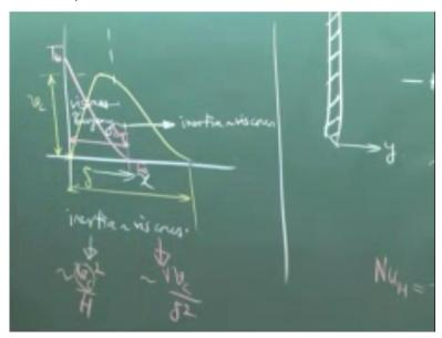
Now we have discussed about thermal boundary layer. But what happens for the hydrodynamic boundary layer. So, let us try to make a sketch of the phenomenon, the velocity and the temperature profile. So, this is x, so how will the velocity profile look? So, the velocity at the wall will be zero and then because of buoyancy effect the velocity will go up an again in the fast stream the velocity will come down to zero, seem critical.
