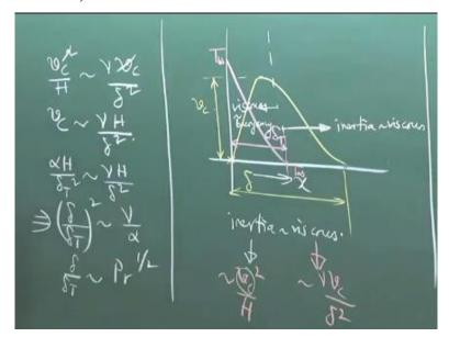
So, these two forces, now if they come of the same order of magnitude, vc square by H is of the order of new vc by delta square, so vc is of the order of new H by delta square and vc is alpha H by delta T square. So, delta by delta T square is of the order of nu by alpha. That means delta by delta T is of the order of Prandtl number to the power half, right? So, this picture diagrammatically is justified.
