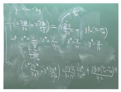
So, to do that we will first not considered the analysis of these equations but we will just nondimensionalised the equations. So, let us write the y momentum equation again. This is the equation. So, our first objective before making any analysis is to ask ourselves a question that, which mechanism of convection is important? Is it force convection that is important, is it natural convection that is important, given a practical scenario.
