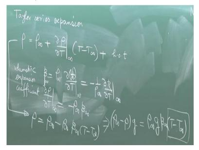
So, you have to make some mathematical analysis to tract these rho as a function of temperature. So that is often done by expanding rho, about rho infinity using a Taylor series expansion as a function of temperature. So, let us do that. So, if the temperature difference is larger and larger, the higher rod at tone terms will be more and more important. But if the temperature difference is not that large, only up to the linear term may be good enough.
