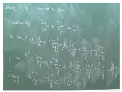
That will be one of the objectives of our further investigation. So, we will try to figure out, so let us figure out the governing equations; let us say that it is a 2-dimensional incompressible flow, so when I am telling that it is incompressible flow, you can pounce on me immediately and say that on one side, you are saying density is changing, on another side, how can you say that it is a incompressible flow? Right?
