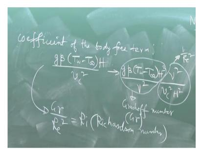
So, if, force convection effects are present, so coefficient of the body force term, let us write; coefficient of the body force term, so theta is the dimensional, sorry; dimensionless parameters, so it varies between 0 to 1. So, its coefficient is, its coefficient is the factor that decides that how strong is that term? So, g beta T wall –T infinity/; there is a H; there was a H, so we multiplied by what? There is a H, right. So, g beta T wall – T infinity/.
