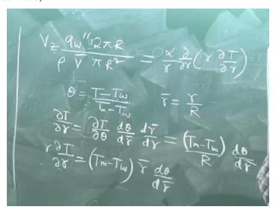
So, you can write this as V z into q double dash. P is 2 pi r perimeter of a circle for is 2 pi r divided by m not is rho into V average into A pi r square is equal to alpha into 1 by r del del r of r del T del r. Now, we will define theta is equal to T minus T wall by T m minus T wall and
