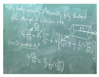
So, anyway now move onto the other geometric which is the circular pipe. Hydrodynamically and thermally fully developed flow through a circular pipe. So, we have now seen the parallel plate channel situation just now we have seen, now will see the circular pipe. So, the concept wise, there is absolutely no difference only the mathematics wise, it will be little bit different which we will see that what different it is
