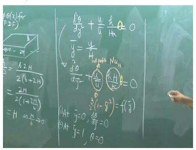
Whatever was in the previous case that was d T m d x, now it will be theta d T m d x. So, here it will be theta, so this will be theta. So, the governing equation instead of d 2 theta d y 2 plus Nusselt number into u by u average, it will be d 2 theta d y 2 plus Nusselt number into theta into u by u average. So, when this theta multiplier has come but this theta multiplier will spoil the ability of this problem to yield an analytical solution.
