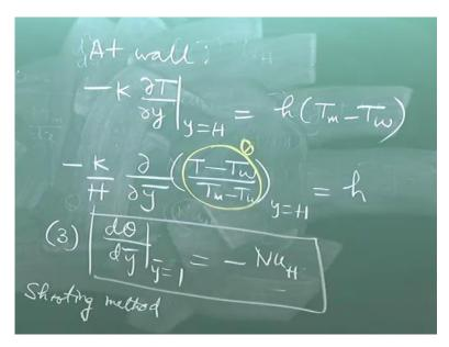
So, you have these 2 boundary conditions on the top of that at the wall, so you have this is the boundary condition at the wall, so you can write minus K del del y bar by H. So, what is this term in the bracket? This is theta, right. Can we write instead of partial derivative and ordinary derivative here? Yes, we can write because for thermally fully developed flow, theta is not a function of x. Theta is a function of y only.
