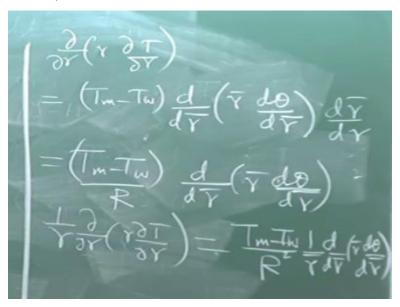
Changing the basis from T2 theta and r2 r bar. So, del T del theta is T m minus T wall and d r bar d r is 1 by R. So, what is r del T del r then what is del del r of r del T del r. So finally, 1 by r del del r of r del T del r. right. T m minus T wall by r square into because this r you can write r bar into R So that R into this R makes it R square.
