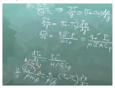
So, now let us look in to this derivation, so this does not depend on whether it is constant wall heat flux or constant wall temperature, d T m d x expression this also does not depend on whether it is constant wall heat flux or constant wall temperature. So, in the governing equation when we have substituted d T m d x. Now in this governing equation you have an extra theta multiplier with d T m d x.
