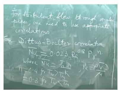
So, for turbulent flow through circular pipes; one need to use appropriate correlations. So, in this correlation the value of this, so again you see the Nusselt number is of the order of Reynolds number to the power n into Prandtl number to the power n. So, that fundamental understanding still remains. Now this Prandtl number to the power n, value of n depends on whether it is heating or cooling.
