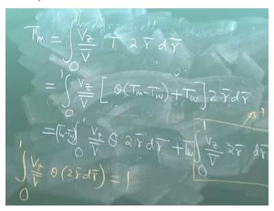
What will this last term? Remember integral of V z into 2 pi r d r is equal to V average into pi r square. So that is the nondimensional form of that ratio which becomes 1. So, that integral of Vz into 2 pi r d r by V average into pi r square that ratio is 1. So, you see I am trying to generalize it, it does not depend on what is the velocity profile, this becomes always 1. So, you can write integral of V z by V average into theta into 2 r bar d r bar 0 to 1 that is equal to 1.
