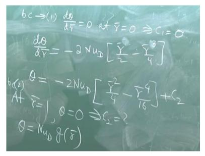
So, boundary condition 1, d theta d r equal to 0 at r equal to 0 that will tell you C 1 equal 0. So, d theta d r is equal to minus 2 Nusselt number into r square by 2 minus r 4 by 4 divided by r that is r by 2 minus r cube by 4, right. Then, we can right boundary condition 2 at r equal to 1, what is theta? Theta is T minus T wall by T m minus T wall, r equal to 1 means wal, so theta is 0. So, these will give you what is C2.
