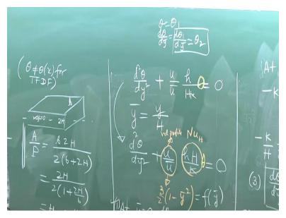
So, you can assume that theta is equal to theta 1 and d theta d y that is d theta 1 d y is equal to theta 2. So, you will get theta 2 as a function of theta 1 and another equation this one. So, these are the two coupled first order. One is d theta 2 d y plus f into Nusselt number into theta 1 equal to 0, right and the other equation is d theta 1 d y is equal to theta 2.
