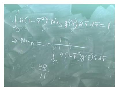
So, V z by V average is 2 into 1 minus r bar square then theta is Nusselt number into g of r bar into 2 r bar d r bar equal to 1. So, that means Nusselt number is equal 1 by integral of 0 to 1 4 into 1 minus r bar square into g r bar into r bar d r bar, right. So, this is the number once this is the simple polynomial integration, there is no trick in this integration because this is a simple polynomial.
