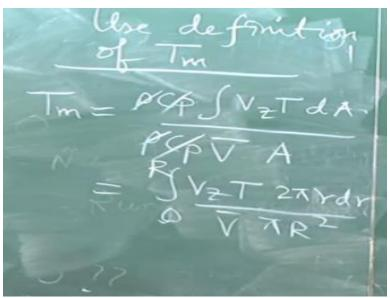
Now how do you calculate the Nusselt number just like the parallel plate channel case, we will use the definition of bulk mean temperature, so use the definition of bulk mean temperature. So,
