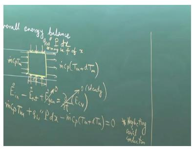
So, let us say that this is the channel and we take a control volume like this. Across this control volume, we are going to write an energy balance, so when we are going to write an energy balance, there is some energy that is entering. Let us say that this length is d x. There is some energy that is leaving, so what is the energy that is entering in terms of the bulk mean temperature.
