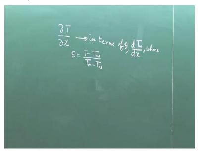
So, for constant wall temperature it is theta into d T m d x and for constant wall heat flux, it is just d T m d x without involving theta that much we discussed in the previous class. Now, irrespective of the boundary condition, this parameter is always involved. So, one thing we have been successful in reducing the dimensionality of the problem that when we are expressing delta T delta x in terms of d T m d x.
