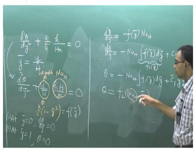
So, we can write d 2 theta d y 2 plus u by u average into h by H K equal to 0, right. Now you can non-dimensionalize like this, right. You can define a new parameter y bar as y by H, ok. So, if you define a new parameter y bar as y by H then this will be d 2 theta d y 2 plus u by u bar h H by K is equal to 0. So, there will be a 1 by H square here that H square coming here will make it h H by K.
