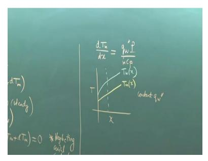
So now from this equation, you can write d T m d x is equal to q double dash P by m dot C p. Now, can you tell from here that d T m d x is constant if wall heat flux is constant, yes or no, yes. Because for steady flow rate is m dot is constant, we assume that the properties are constant then the perimeter of the cross section, it is the constant for the geometry that we are considering. So, if the wall heat flux is constant then the d T m d x is constant.
