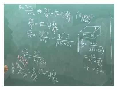
So, similarly the second derivative and what is d T m d x, d T m d x is what is that expression q double dash P by m dot C p, so q double dash in place of P, let us draw a parallel plate channel. Let us say that the width is b and height is 2 H with the center line is y equal to 0. So, what is the perimeter, so before that let us write another step. What is m dot, m dot is rho u average into A into C p by perimeter.
