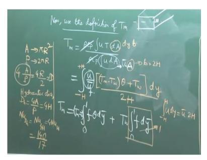
So, what is the area, area is pi r square. What is the perimeter 2 pi r, so what is area by perimeter? So how can you get diameter from here, multiply by 4, so these becomes diameter, ok. So, 4 into area by perimeter for a circular pipe is the actual diameter. For a noncircular geometry that is some effective diameter which is called hydraulic diameter. So, hydraulic diameter let us write it here is 4 into area by perimeter.
