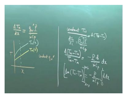
Now, this is the case of constant wall heat flux. Let us stud y the qualitative behavior of constant wall temperature may be first we studied quantitatively and then we show it in a plot. So, the case of constant wall temperature. So, d T m d x is equal to q double prime p by M dot C p. How can you write q double prime in terms of the heat transfer coefficient h, q double prime equal to what h, h into T m minus T w or T w minus T m.
