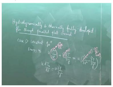
So, hydrodynamically and thermally fully developed flow through parallel plate channel. Case 1, constant wall heat flux. So, what answer can we expect for these types of problems. What are you assured of when you are solving a problem of thermally fully developed flow. We are interested about the Nusselt number. The Nusselt number will be a constant that is what is expected.
