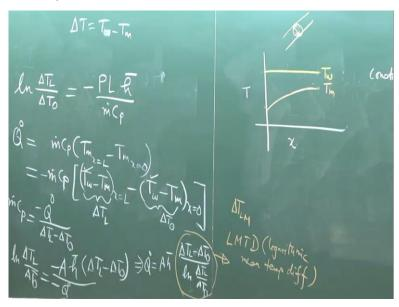
So, we can write Ln of delta T L by delta T 0 where delta T is T wall minus T m is equal to, so what is this, this is the average heat transfer coefficient times L. So, minus P into L into h average by m dot C p. Now what is the total heat transfer rate, Q dot. Let us say you transfer some heat from the wall to the fluid, so how can you measure what heat has been transferred from the wall to the fluid.
