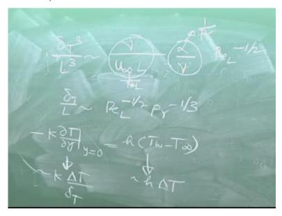
So delta T cube/L cube is of the order of; alpha/ u infinity L means u infinity L / nu, we put the nu in the numerator \* alpha/ nu, right\* Reynolds number to the power of -1/2. So this is what? This is Reynolds number. Yes, 1/Re and this is 1/Re Prandtl number. So delta T/L is of the order of Reynolds number to the power of -1/2 \* Prandtl number to the power of -1/3, right.
