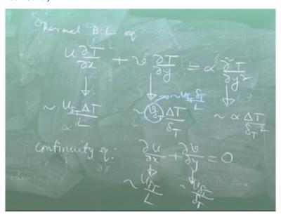
So thermal boundary layer equation; what is this? this is v at delta T. Now we will use the continuity equation. So this is of the order of; remember we are interested within the thermal boundary layer. So u delta T/L, this is of the order of v delta T/delta T, that means v delta T is of the order of u delta\*delta T/L. Again, the same conclusion that these 2 terms are of the same order.
