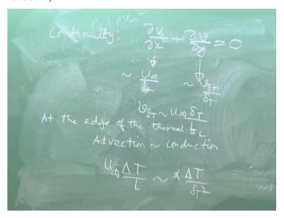
What is the order of magnitude of this? This equation is analysed within what? Within thermal boundary layer, because our objective is, you can analyse the continuity equation both within thermal boundary layer as well as within hydrodynamic boundary layer. But you
