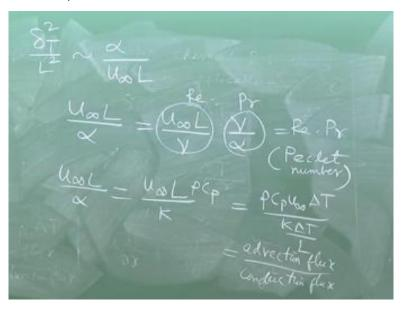
So at the age of the thermal boundary layer; that means we can write, so delta T square/L square, we can write u infinity L/ alpha. So what is u infinity L/ alpha? This is u infinity L/nu \* nu/ alpha. Right, So Reynolds number \* Prandtl number. This is also called as Peclet number. Now what does it physically represent? So, u infinity L/alpha, you can write it as u infinity L/k rho, cp in the numerator, right.
