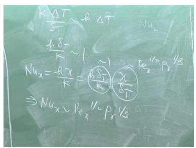
So finally -k del T/ del y at y=0 = h\*T wall- T infinity, so this is of the order of k\*delta T/ delta T, this is of the order of h\*delta T. So we can write k delta T/ delta T is of the order of h delta T, that means h delta T/ k is of the order of 1. This is same as the previous case. So the Nusselt number, that is hx/k = h delta T/k\*x/delta T, which is of the order of 1. At x/delta T is of the order of Reynolds number to the power of 1/2\* Prandtl number to the power of 1/3.
