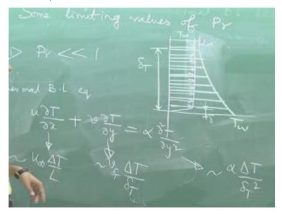
Case 1, Prandtl number much less than 1. So, if you want to draw the velocity and temperature profiles at a given location, Prandtl number much less than 1, always remember that in force convection, Prandtl number has a meaning of delta y delta t. We will see that these meaning may be disturbed, if you have natural convection. We will talk about that in details when we discuss about natural convection.
