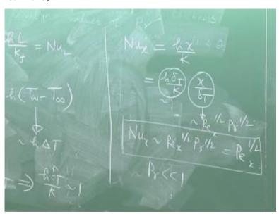
So Nusselt number at a given x, the maximum value of x is x=L, but at any local x, that is = hx/k. This is nothing but, h delta T/k \* x/delta T. h delta T/k is of the order of 1 and x/delta T; you can see here, just think of L replaced by x, Reynolds number L will be replaced by x. It will become local Reynolds number. So x/delta T will be Reynolds number to the power of 1/2 \* Prandtl number to the power of 1/2.
