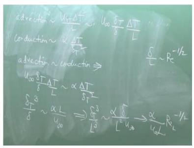
So we can write that advection is of the order of u delta T\* delta T/L, that is of the order of u infinity and conduction. So, we can write delta T cube /L cube, that means we are dividing both sides by L square, so it is alpha delta/L square u infinity. Delta/L, what is delta/L, is of the order of the Reynolds number to the power of -1/2. Delta y/l does not depend on Prandtl number, so this is of the order of alpha/ u infinity L\* Reynolds number to the power of -1/2.
