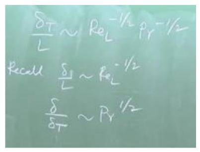
So, what is this? This is advection flux; this is conduction flux. In convection, what we are always trying to see or explore that how is advection enhancing or augmenting the heat flux with only conduction, there would have been some heat flux, with advection, how that can be augmented, that is one of the big objectives of studying convection. So you can write delta T/L is of the order of Reynolds number to the power of -1/2 x Prandtl number to the power of -1/2.
