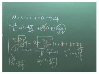
Dh/Dt equal to Cp DT/Dt plus. So, in the left-hand side what is required is rho, you multiply by rho all the terms. So, when you multiply all the terms rho into specific volume is equal one. Now you compare the left-hand side and right-hand side of this energy equation and we can observe one very interesting thing that this Dp/Dt and this Dp/Dt they get cancelled from both sides, right.
