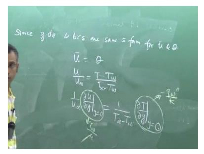
Is u/u infinity equal to T minus T wall. Again, I am repeating that as an engineer we are not so much bothered about what is a temperature? What is the velocity? In fluid mechanics, what is the most important parameter the wall sheer stress that we are bothered about. And in heat transfer what is the most important parameter wall heat flux. So, wall sheer stress in fluid mechanics and wall heat flux in heat transfer.
