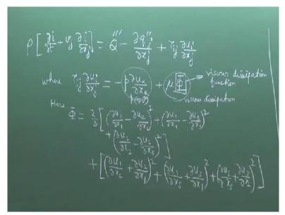
That equation is written here with i as the internal energy so various terms this is like the total rate of change of internal energy. This can be attributed to volumetric heating, surface heat flux and viscous dissipation. So, one part is viscous dissipation and this is pressure work or PDVP, P dot delta v, sorry p into delta dot v. So, p into Delta dot v that term is there which is just like the PDV work in thermodynamic. So, this is due to volumetric change whatever is the work done.
