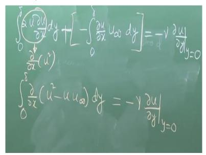
So, that will become integral of 0 to delta, 2u del u/ del x dy+ in place of v infinity, we will write -del u/ del x dy. So, this can be written as del del x of u square, right. So, if you now consider these two terms together, it will be integral of 0 to delta, del del x of u square -u u infinity dy, okay. Now the next question and this is the very important question, can we bring these derivative out of the integral.
