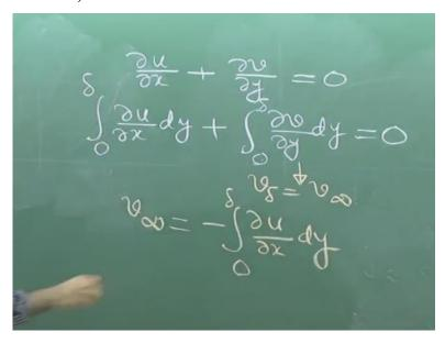
Now there is still unknown in these equation which is v infinity, so we will try to obtain a v infinity by using the continuity equation. We will integrate this equation with respect to y. So, what is this? This is v at delta - v at 0, -v at 0 is 0. So, v at delta is v infinity. So, v infinity= integral of del u/ del x. So, this v infinity, we can substitute in this equation. So, in this equation, we will substitute the v infinity, which we got from the continuity equation.
