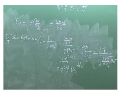
So, that is remembered u/ u infinity is (3/2 y/delta-1/2 y/delta) cube. So, toe wall is 3 mu u infinity/2 delta. Normally, the wall shear stress is expressed in a non-dimensional form by using these non-dimensional parameters cf, which is called as skin friction coefficient. This is toe wall/ 1/2 rho u infinity square and delta is, what is delta? Delta is square root of 3 nu x/au infinity.
