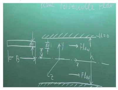
But physically it is not so because the flow takes place in this direction, this is the flow direction. So, shear stress at the lower plate is acting in this direction and the shear stress on the upper plate should act also in this direction. So where is the problem, where is my confusion. This is because the coordinate, the upper plate implies that tau x y is opposite to that. A positive tau x, y is in the opposite direction.
