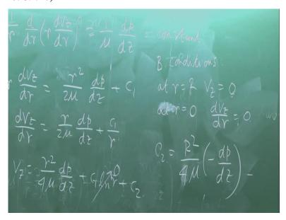
And here also the boundary conditions are at r is equal to r vz zero. We have two constant. Another boundary condition is the azimuthal or axi symmetry condition which means dvz dr at r is equal to zero, rather you write in the same fashion, r is equal to zero, dvz dr is zero. Okay? And this automatically says that this equation cannot have a term like this, lnr is, that
