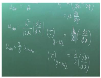
Now shear stress here takes place in the direction of x at any plane which is perpendicular to y whose normal is in the y direction. So, tau xy from a general relation we know mu multiplied b shear rate or rate of angular or shear strain in xy plane, that is del v del x plus del u del y, but at this moment, this is not necessary because we know everything here that there is no free component and U is a function of u y only, du dy.
