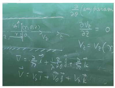
And in a cylindrical coordinate system I write the divergence is as you know is del del r, ijk if vr v theta, now I have to define vr. vr is this, in the r direction. Vz is along vz direction and v theta is along the theta direction. So therefore, this is one up on r del del theta j plus del del j k and v the velocity vector is defined as vr i j k are the unit vector v theta, sorry and vz k. Now this is a preliminary vector calculus.
