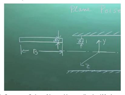
Now volumetric flow rate to find out, I have told you earlier that if I take a small element dy here and if you consider its width as b, a small element like this, cross sectional plane, that means if you see this view it is like this. This is dy and this is d. That means if we consider a small element of height dy and width d then through that the flow rate is du multiplied by B dy. That is the value of u prevailing at that particular y.
