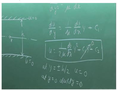
Now in general, we have already developed that in Cartesian coordinate system, for this situations of exact solutions our Navier-Stokes equation becomes d square u d y square, this already we appreciated 1 by mu dp dx. V0 w by definition 0, there is no velocity in the jet component and the width of the channel is so large compared to this spacing or the height and here we define this as h, total spacing, that the change of any parameter with respect to J is negligible compared to X and Y.
