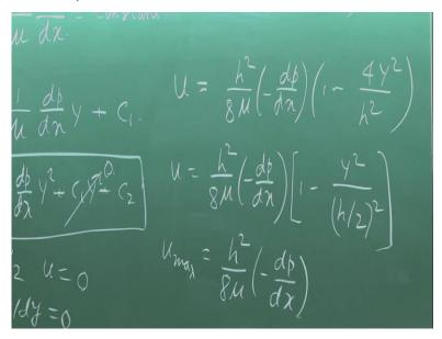
And if put this boundary condition we get, c2 is equal to h minus 1 by 8 mu. I write 8 square by 8 mu minus, this is a style of writing minus dp dx, so c2 becomes h square by 8 mu minus dp dx. So, if you substitute this c2 here, finally you get the velocity profile like this, h square and h mu you take this as common, minus dp dx into one minus 4 y square by h square. If we just put the value of c2 here.
