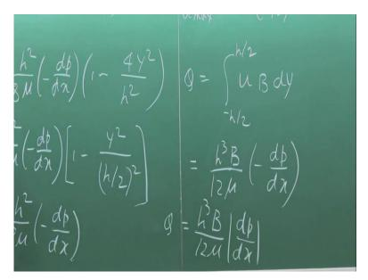
So sometimes we can write that u by U max this is another way of representing is one minus y square by h by 2 whole square. This is the velocity distribution. The next task is to find out the volumetric flow rate Q.
