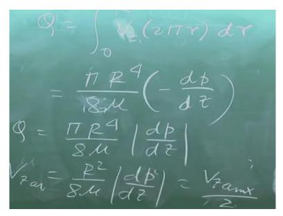
And to represent the q you can express this as the modulus of this. That means Q can be expressed as pie r four by 8 mu. I think this is more reasonable to understand because volume flow rate has no sign and vz average therefore is equal to then divided by the cross-sectional area, that means r square by 8 mu multiplied by dp dz which is vz max by two. Now I come to the coefficient of friction.
