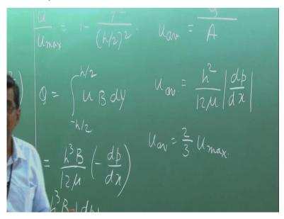
U average as average velocity in fluid flow is defined by the volumetric flow rate. That means for internal flow, flow through a duct, is defined as volumetric flow rate divided by the cross-sectional area. And if you do that cross-sectional area is B multiplied by h, then you get h square by 12 mu mode of dp ds. Of course, here you can put that minus dp dx type of thing to show the direction of Uaverage which will be inconsistent with the direction of U.
