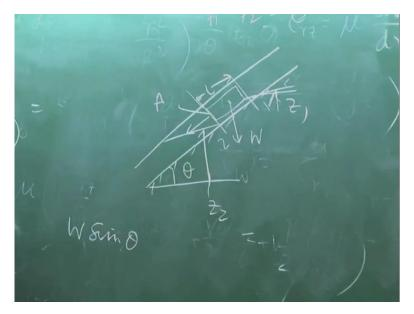
For an example if there is an inclined plane and liquid plane is flowing and this plane is inclined by an angle theta. So, if you take a fluid element, pressure here is all atmospheric at this and this. If this is section one and this is section two, p1 minus p 2 is zero, but then what causing the flow is the gravity, that means the component of its width in this direction and that is the difference of the piezoelectric pressure force.
