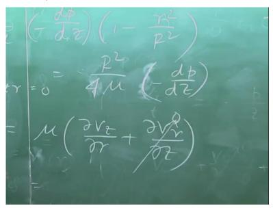
Next task is tau w which is tau rz. First of all, let us write tau. That means shear stress in the direction of flow which is in the rz plane. At any plane parallel to the flow that is rz plane which can be written as mu into corresponding rate of angular or shear strength, that is del vz del r plus del vr del j. This has been taught at your basic fluid mechanics class, since in this case vr is not there and vz is a function of r.
