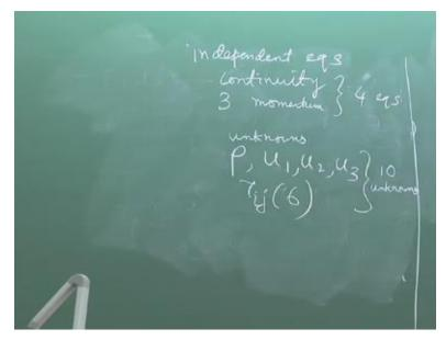
Independent equations, how many equations one is continuity equation. The second is you have this equation for three components so three momentum equations. So total four equations. Unknowns, what are the unknowns? In general, you may have rho as an unknown, density may be unknown then u 1, u 2, u 3 then six components of tau i, j body forces usually prescribed it is know because you are interested about the motion given a particular body force.
