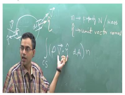
Let us make a sketch of the control volume, let us say this is an outflow boundary. Let us say dA is that elemental area on the outflow boundary. Let us say that V is the velocity of flow at this outflow boundary. And small n is the property N / unit mass. We also describe a unit vector, normal to the perceive. Let us say that Eta is a unit vector, which is, so what is Eta, unit vector normal (outward) normal.
