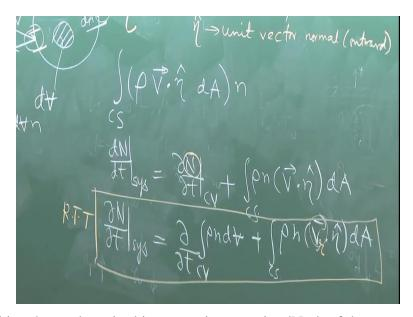
So, we can combine that and use in this expression to write dN, dt of the system. What is capital N of the control volume? Let us say this is a small element dC, a volume element that we get. What is the mass of this element? Rho \* dV. What is the property for unit mass? Small n. So, the total property is this \* small n.
