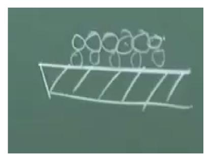
Let us say this is a wall, the first molecule, which are adhering to the wall will directly feel the effect of the wall so if the molecules are significantly compact, then they are almost like trapped by the attractive interactions of the wall and they cannot escape from the wall. This in fluid mechanics, in classical fluid mechanics is known as no sleep boundary condition. There is no relative tangential component of velocity between the fluid and the solid boundary.
