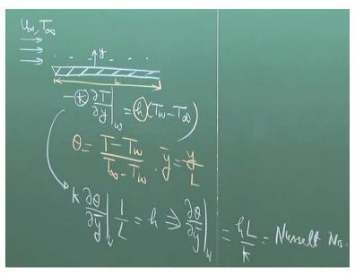
Let us say that you have a solid boundary and fluid is coming from fast stream with a velocity U infinity and temperature T infinity. Now, to write what is the heat transfer at the wall, we express it by this following boundary condition. We have discussed earlier that this boundary condition
