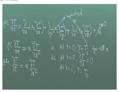
So, this slab is much wider and much longer in height as compared to the thickness. So, the gradients along y and z directions are neglected. This is also neglected. If these are neglected and
