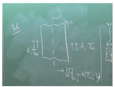
Let us say same infinite slab. Let us say that some fluid is flowing outside the slab with heat transfer coefficient h, and temperature T infinity. So, the only difference from the previous problem is that there is a different boundary condition. Previous problem what type of boundary condition it was? It was a Dirichlet type of boundary condition where the temperature was specified. What type of boundary condition is not there for this problem?
