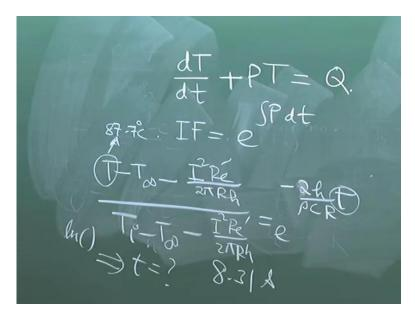
Now what will be the unsteady state variation because for the second problem basically we require to find out temperature as a function of time, right. So, if you look into the differential equation. The differential equation is of this form right, where P and Q are some coefficients. This is the form of the differential equation. So, for solving this differential equation, we have to multiply with an integrating factor e to the power integral P d t.
