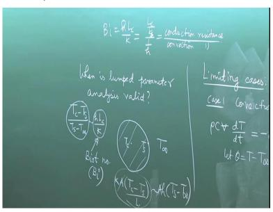
So, let us take this example. Let us say that you have a spherical ball with T c as the centile temperature, T s as the surface temperature and T infinity as the temperature of the surrounding fluid. This is a solid ball. So, you can write not exactly equal because it is not a steady state problem, so the heat transfer due to conduction is not exactly minus K a into delta T by L.
