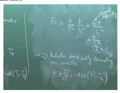
So, how do you define Fourier number? Fourier number where alpha is the thermal diffusivity. Alpha is K by rho C that is the thermal diffusivity. So, this can be written as T by
