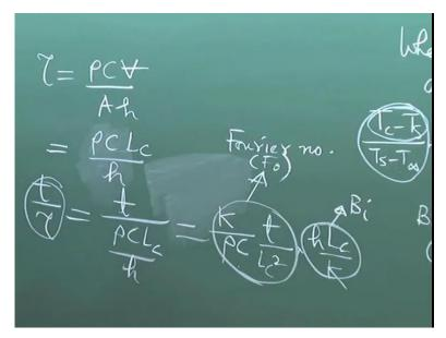
So, when you go for purchasing of a temperature measuring instrument you should look into the time constant and make sure that the time constant is small. Then how can we write this A h by rho C v into T, so you can just manipulate the algebra and you can write T by tau in this way. So, T by tau is T by rho C into L c by h, L c is viva A, ok. So, now you can multiply by K. Why you multiply by K? because you want to get the Biot number.
