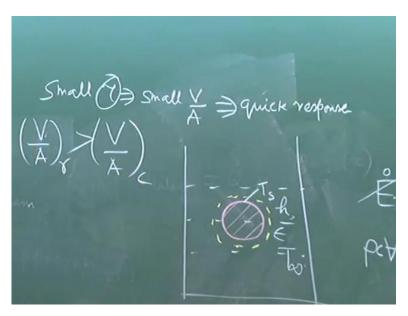
So, if the riser must lose heat most slowly then the time constant of the riser must be large, right. That means volume by area of the riser must be greater than volume by area of the casting because its time constant should be large so that it should respond slowly to the thermal change so that it will not immediately freeze. This in riser design problem is known as (()) (15:00) rule.
