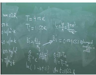
So, the first problem, please note down the problem. This is a problem from incropera book. Steel balls of 12-millimeter diameter, so D is equal to 12 millimeter, this is 2 R or annealed (annealed means annealing is a heat treatment process) by heating to 1150 Kelvin and then slowly cooling to 400 Kelvin. I am repeating steel balls of 12-millimeter diameter or annealed by heating to 1150 Kelvin and then slowly cooling to 400 Kelvin.
