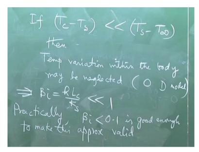
So, we can write if T c minus T s is much much less than T s minus T infinity then temperature variation within the body may be neglected. This is zero-dimensional model. So, the model is valid see you cannot adjust this (()) (7:47) because you do not know what are the temperature, so you cannot put this values and check. So, what you can check? You can check this parameter.
