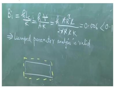
First of all, before applying the unsteady state situation can we use the lumped model here? So, let us say that length of the wire is L. So, the Biot number h R by 2 K, ok. So, if you substitute these properties this will be 0.006. This is less than 0.1. So, it a sufficient condition for the lumped parameter analysis to be valid. So, now let us try to make a control volume analysis of this electrical wire.
