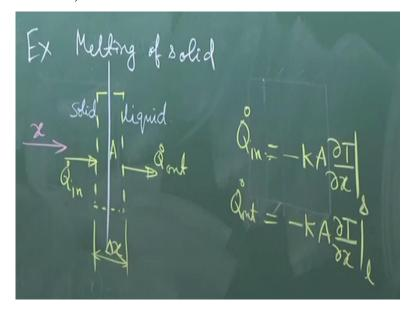
So, we are taking an example which is little bit different this is melting of a solid. So, let us say there is a solid, there is a heat transfer here, let us say it is a 1-dimensional situation. There is a heat transfer along x, so some heat is utilized for melting the solid to liquid. Let us say that we take a small control volume like this surrounding the interface. This control volume is of thickness delta x in the limit as delta x tends to 0 we can recover a sharp interface.
