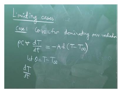
So, limiting cases: Convection dominating over radiation. Now, you can solve this equation. Let us say that theta is equal to T minus T infinity. So, you can write d theta by theta is equal to minus A h by row CV d t. So, if you integrate this ln theta is equal to minus A h by row CV t plus ln C1 where ln C1 is a constant of integration. So, theta is equal to C1 into e to the power minus A h by row CV t.
