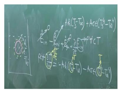
Let me give you an example, let us start with an engineering example, in manufacturing or in processing of materials, there is a process which is called as quenching. Quenching is a heat treatment process, so in quenching what happens let us say you have a metal block which you had heated, so heat treatments are done in materials industry to give sudden material property to impart certain properties to the material.
