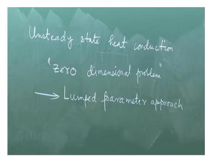
Now, we will move on to unsteady state heat conduction. When we think of unsteady state heat conduction, the situation is that we are considering that temperature is also a function of time. So, as I told you earlier that all problems are fundamentally unsteady so we are doing unsteady state analysis when our time domain of interest is such that over that time domain temperature is changing with time.
