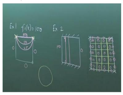
Example 2, let us say these 2 boundaries are adiabatic. When you have adiabatic boundaries, you will have constant temperature line perpendicular to the boundary and the reason is obvious. If it is adiabatic then what does it mean it means that the heat flex is 0 that means the normal temperature gradient is 0 that means along the normal direction temperature is not changing. Therefore, the normal direction is the isotherm or constant temperature line, ok.
