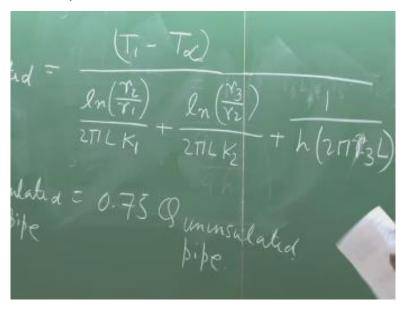
What is the Q insulated pipe = their subjective to same potential difference because environment remains same and the inside surface remains same, Q1-T infinity, very simple problem, heat transfer until and unless you come to convection, heat transfer things are very simple as far as this your under-graduate level material is concerned, how about conduction contents, high level mathematics after watts 3-dimensional conduction unsteady state.
