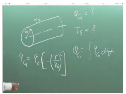
Now the problem states like this, I am telling if there is a cylindrical container, this is the axis; cylindrical container of radius r0 and the language of the problem is like that radioactive Os are packed in a long thin wall cylindrical container, that means the radioactive Os are packed that means ultimately works as a solid cylinder type of thing. The radioactive Os are packed in a long thin wall cylindrical container.
