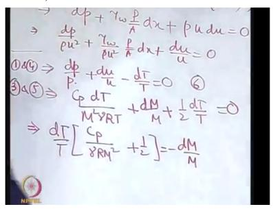
So from this expression it is possible to express dM/M as a sole function of dT/T involving the Mach number or dT/T as a sole function of dM/M as a function of Mach number. So if you take dT/T common we have Cp/gamma RM2 then + 1/2 = - dM/M, so this mean that we have dT/T = - dM/M/Cp/gamma RM2 + 1/2. Let us give it an equation number 7.
