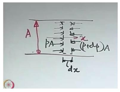
The next fundamental equation that we may think of is momentum conservation. So let us try to write the momentum conservation equation, to do that let us consider a control volume of width dx. The pressure acting on one side of the control volume is P so the force is P \* A,
