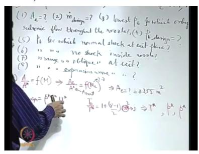
First of all, what is the area of the exit. So to know that if we refer to A/A star, we know that A/A star is the function of Mach number only. This we have derived earlier, so based on that we can find out what is Ae because the Mach number at the exit is given which is 2.7. A star is nothing but area of the throat because the sonic condition here is reached at the throat so from here we can get what is the value of Ae which is 0.255-meter square for this problem.
