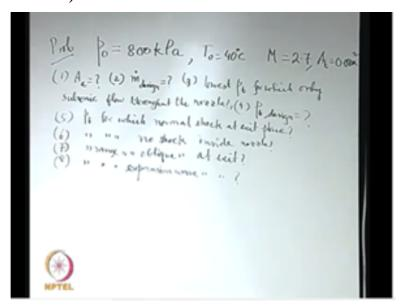
The problem is as follows; a convergent-divergent nozzle is designed to expand air from a chamber in which P0=800 kPa which is the stagnation pressure. T0=40 degree centigrade to give the Mach number equal to 2.7 at the exit. The area of the throat is 0.08-meter square this is the given data.
