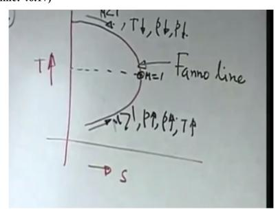
So the upper part corresponds to a subsonic flow and the lower part corresponds to a supersonic flow and these parts go through a point of maximum entropy where M=1, so this
