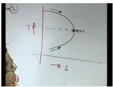
Now what are the differences when you are having the process which is going towards the maximum entropy which is the natural spontaneous way by which a process may thermodynamically take place, but there are 2 different parts by which one way reach that process for this case. For the part above if you look into it very carefully we will see that as it
