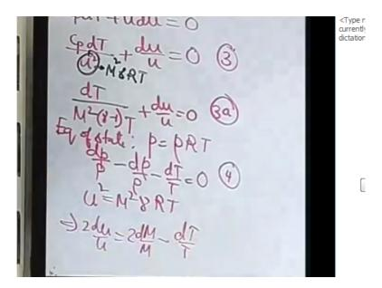
We will have a further simplification of equation number 3 or maybe you will call the next step as equation number 3 so CpdT/u2 +du/u = 0 by dividing by u2. Remember that u2 is nothing but M2 x gamma RT and accordingly we may write in the next step that using CP/R is gamma by gamma -1 so this becomes dT/m2 \* gamma -1 in T + du/u = 0, let us say this is equation number 3a.
