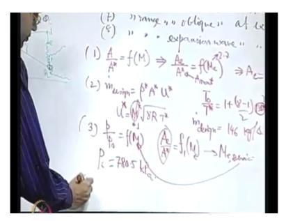
So we can find out this one to be equal to that is the pressure at this point C as 780.5 kilo pascal. Part 4, what is the design back pressure? The design back pressure you may calculate exactly in the same way as part 3, but you replace the subsonic solution with the supersonic solution, so here M corresponds to the supersonic solution that is 2.7 that is the back pressure that is pressure at the point g in the figure by P0.
