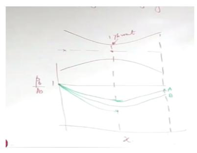
So, for the converging diverging nozzle, let us say that you have a nozzle like this which has a converging part and a diverging part, so if you refer to the expression for dm/m, you can clearly see that for m > 1, dm/m is > 0, if dA/A is > 0, that means it is possible to have an increase of Mach number from the critical case, which you may come here as m = 1, so this part is just like a converging nozzle, so the critical condition that you may achieve here is m = 1.
