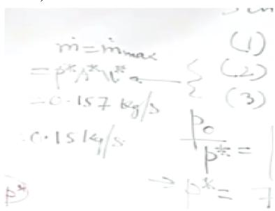
That means, the saturation in the mass flow rate has already been achieved and therefore, for calculating the mass flow rate you should not go through this route but it should go through the m dot max route, so for both 2 and 3, you have m dot = m dot max, this is rho star A star \* u star which we have just derived. So, this you can write exclusively in terms of the stagnation properties in terms of P0 and T0
