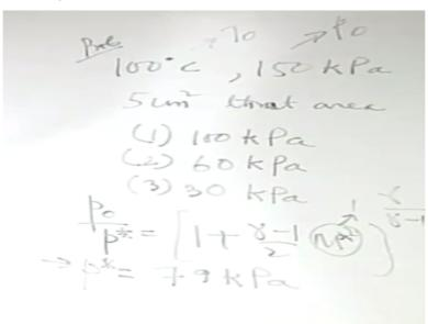
So, the problem statement is like this; here in a large tank at 100 degree centigrade and 150 kilopascal of pressure exhaust to atmosphere through a converging nozzle with 5 centimeter square as throat area; throat area means the exit area for the converging nozzle. Compute the exit mass flow rate, if the atmospheric pressure is; number 1, the atmospheric pressure is like the back pressure is = 100 kilopascal.
