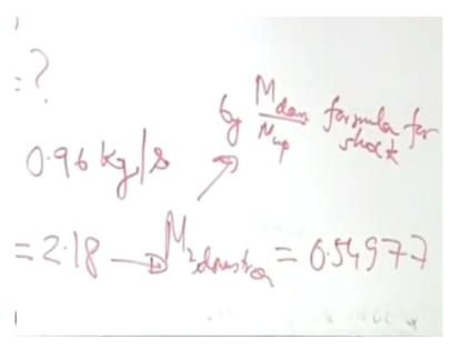
So, M2 upstream; this will give you what is M2 downstream by M downstream/ M upstream formula for shock that is M2 square in terms of M1 square that formula. So, that will give you M2 downstream = 0.54977, when you have got an M2 downstream, you can calculate A2/A2 star downstream.
