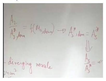
So, A2/A2 star downstream is a function of M2 downstream, so from here, A2 still remains the same, so from here you can get what is A2 star downstream and that is same as A3 star. So, then from this, you therefore have what is A3/A3 star, this is a function of M3. So, out of the possible M3 is again, it has 2 solutions which M3 we will take; subsonic or supersonic? Subsonic because it is downstream of the shock.
