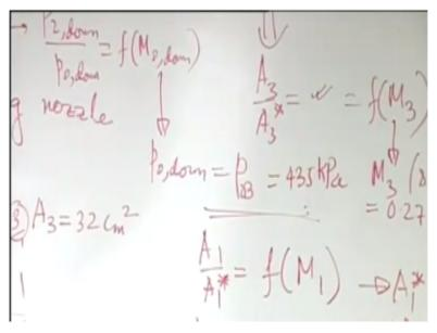
So, P2 downstream/ P0 downstream is a function of Mach number at 2 downstream, which is already calculated. So, from here you can find out what is P0 downstream that is same as P03, okay but if you use the table of shocks, you need not do all these, it is simply given a P0 downstream/ P0 upstream because it goes through all these calculations and eventually tabulates in the form of that.
