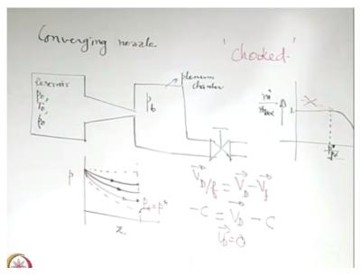
So, we will first start with example of a converging nozzle, we have seen earlier that one of the important objectives that you have with our nozzle is to accelerate the flow and to do that let us say that you have a tank, you connect a converging nozzle with the tank, we have seen earlier that the nozzle shape always did not be converging and in fact, one could have accelerating flow with a diverging section also.
