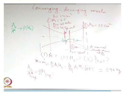
So, with this understanding, now let us try to work out a couple of problems on the converging diverging nozzle. So, the problem is like this; air flows through a duct as shown in the figure, the duct is like whatever is drawn in the sketch with there are 3 sections; section one with given M1 = 2.5, P1 = 40 kilopascal and T1 is 40 degree centigrade, the throat name is section 2, no sorry, throat name is not identified as any section.
