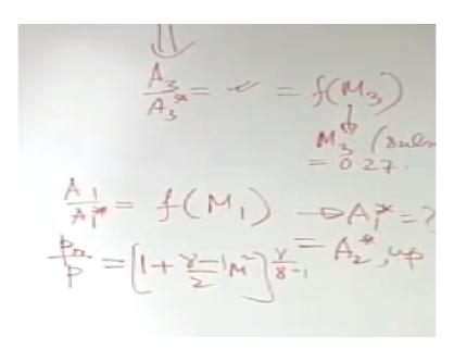
So, this you get what is M3 as the subsonic solution that is = 0. 27 that is the part 2 of the solution. What is the part 3 of the solution, what is P03, so how do you find out P03 that is; yes, how do you calculate P3, how do you calculate P03? This you tell, how do you calculate P03? See, you have P star okay, then so you have P0/P as a function of what; 1 + gamma - 1/2 M2 square to the power gamma/ gamma - 1.
