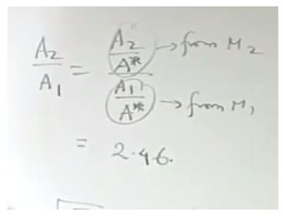
Not only that M is increasing, so from 2 to 2.98, so dM/M is positive, the denominator is always positive that means, dA/A has to be positive, so it is an increasing A, it is a diverging section and how to find out what is the real value of A2/A1? So, A2/A1 is nothing but A2/A star divided by A1/A star, remember what is A star? A star is the equivalent area at which sonic condition could be achieved under an isentropic process.
