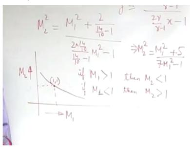
So, air is gamma = 1.4 example, so for air let us write what is M2 square/ M1 square, so M square is = M1 square + 2/ gamma is 14/10 - 1, we will just write it in a fractional form, so what will be M2 square in terms of M1 square? This will be 4/10, so 10 \* 2 in the numerator, 20/4 is 5, so this is M1 square/ 5; M1 square + 5 and this will be 7 M1 square - 1. Now, let us try to make a plot of M2 as a function of M1 from this variation.
