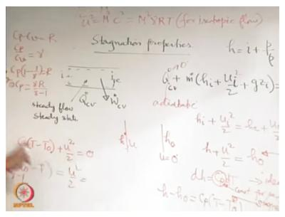
This definition does not require to process to be reversible. So if you want to find out what is stagnation temperature, infect this definition does not require any process because it is just an expression. So if you know the temperature and velocity at a point and specific heat at a point you know the stagnation temperature at a point. So Stagnation temperature is defined at a point irrespective of what is. I mean what kind of state is there at the point.
