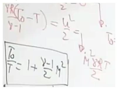
So those properties also you may find out, so for an isentropic flow. For isentropic process you have T p to the power gamma=constant, that means basically in terms of T and P you can write T2/T1=P2/P1 to the power gamma-1/gamma. So just like you have related the stagnation temperatures, similarly you can relate stagnation pressure P0/P=T0/T to the power gamma/gamma-1 that means 1+gamma-1/2M square to the power gamma/gamma-1. Okay?
