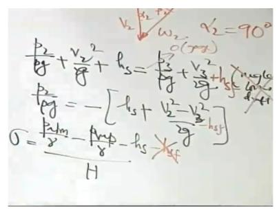
So let us apply the energy equation between 2 and 3. So you have p2/rho g+v2 square/2g+hs=p3/rho g+v3 square/2g. If we neglect any losses neglect losses in draft tube. In reality that is not the case. So p3 is the atmospheric pressure. So if we consider it as a 0 (()) (41:52) pressure. So you can write p2/rho g as - of hs+v2 square-v3 square/2g. Now satisfying the purpose of the draft tube you must have v2 is > v2 right that is for your whole purpose.
