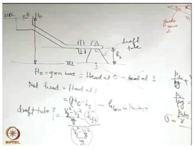
So how it is defined it is defined as draft tube efficiency which is v2 square- v3 square/ 2g-the head loss in the draft tube by this one. Again you see that here what is the purpose? The purpose is in the ideal case the draft tube could recover this amount of energy, but in reality it cannot recover this amount of energy because there is a head loss in the draft tube and that is why it is a efficiency of the draft tube.
