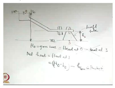
So you have supply reservoir, you have the penstock basically same as for the impulse and the reaction turbine. Then we will draw it very, very schematically to get the picture. This is the head race level this is the tail race level and this is a schematic diagram of the turbine. So you may consider certain points. Let us say that this is section 1 this is section or may be let us call it 0 because it is just the reference.
