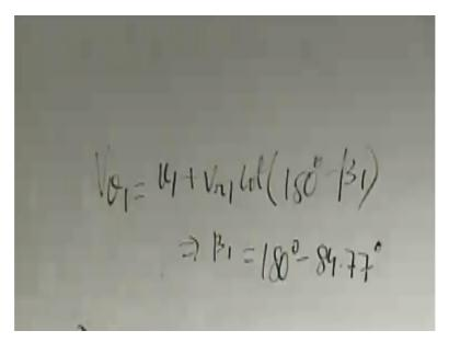
So you can write this one v theta 1 as u1+ Vr cot 180 degree- beta 1. So from here you can find out what is beta 1. So beta 1 is actually in answer 180 degree- beta 1 is given. So beta 1 is 180 degree- 84.77 degree. What is a loss?
