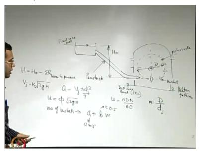
So if you have a nozzle here which is sort of diverting a fluid jet. What is the head that is available with the nozzle that is H0-summation of all the head losses in the penstock. And ideally the nozzle should develop a velocity or the velocity of the jet as what root 2 g H that is the entire head could be converted into the kinetic energy of the jet, but in reality that does not happen because there is some loss in the nozzle.
