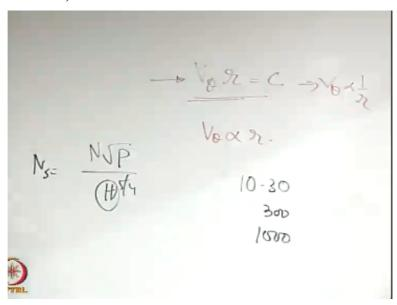
So you have the first requirement is when it is entering the flow passage you have v theta \* r= constant. So you have this v theta \* r= constant that is when it is entering the flow passage. Now on the top of that you have to keep in mind that when it is entering the runner you have v theta is proportional to r it is like v=omega r type. So when it enters the runner you should have v theta proportional to r here v theta is proportional to 1/r before just entering the runner.
