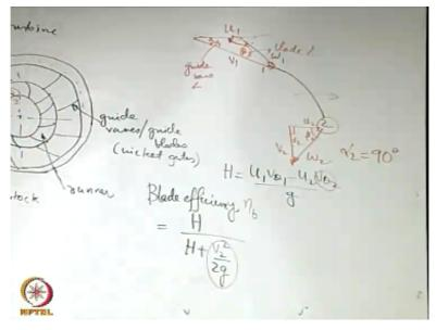
When the jet falls on the rotating blades let us try to construct velocity triangles and see that what happens. So you have this as say 1 and this as 2. So the points 1 and 2 just very much analogous to centrifugal pumps only the reverse flow direction. So you have say this is as U1 and this is w1 and this is v1. Let us say that this is beta 1 and let us say this is alpha 1. What is the physical importance of the angle alpha 1?
