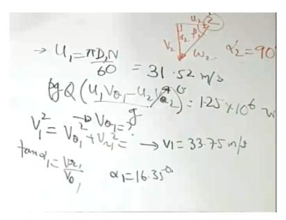
So you have first of all you can calculate U1 that is pi D 1 N/60. So I am just giving you the numerical answer so that you can check 31.52 meter per second. Then the power developed is rho g Q\*h. H is U1 v theta 1- u2 v theta 2/g that is given as 12.25 megawatt 12.25 \* 10 to the power 6 watt. It is given that the flow leaves without whirl that means v theta 2 is 0. So this is one information that is given.
