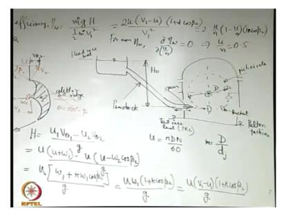
So let us consider w 2=k w1 so this here if you take u common this is w1+ k w1 cos beta 2/g. So u \* w1 \* 1+ k cos beta 2/g. You can write w1 as again v1-u. So u \* v1-u \* 1 + k cos beta 2/g. For impulse turbines there is a particular terminology called as wheel efficiency. Usually hydraulic efficiency is used wherever you have pressure change as well. So here you just have some energy change based on the input form of energy which is the kinetic energy form.
