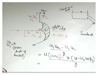
So if you consider if you draw the bucket in the way in which it is facing the fluid it is something like this. So this is the bucket the water is coming from this side. It is interacting with the bucket and the bucket is deflecting it. So actually the water jet which is coming is getting split into 2 parts and there is something there is a particular structure which allows it to split it into 2 parts. This is known as a splitter ridge.
