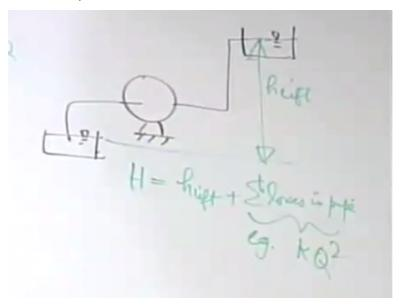
The operating point is the point where the head supplied by the pump is just good enough to achieve this lift and to overcome all the losses in the system. So that will be the point of intersection between the pump and the system characteristic right. So this will be the operating point and the operating point definitely is going to be different from the design point.
