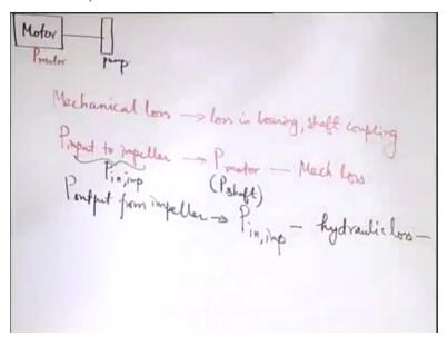
So if you recall that schematically we may consider that you have a motor which is the sort of driver for the pump. So there is a shaft and on this shaft is mounted the impeller of the pump, so you have this as the pump so to say just schematically we may call this as a pump and then there is some energy output from it. So let us just look into it in the form of the power or energy transfer.
