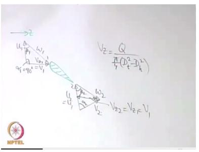
So that is=u2-vz2 cot beta 2 right. This angle is 90 degree so you can clearly write it from the trigonometry and vz2 is like you have this as same as Q/pi/4 d tip square-d hub square okay. So that means how will the power depend on beta 2? So if you increase beta 2 what will happen cot beta 2 will increase or decrease. It will decrease and therefore we expect that the head should be more. So you will have a temptation of increasing beta 2.
