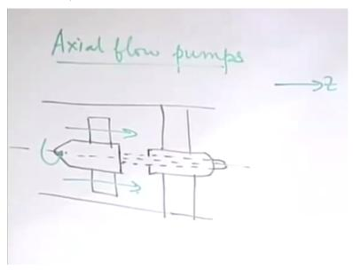
What is that? This is pi/4 diameter of the tip square-diameter of the hub square. So this is the hub and this is the tip okay. So in this passage there are blades and the fluid is flowing. So then this one see the diameters of the tips and hubs are not changing as you are going from from the inlet section to the outlet section. The flow rate is also not changing, so you expect vz also to be the same.
