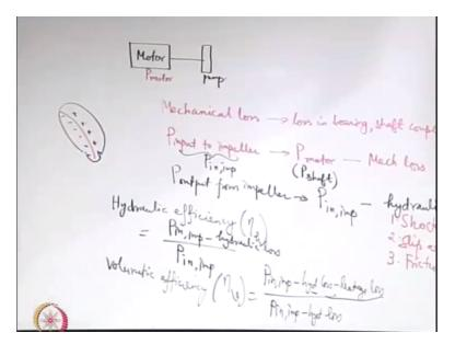
So hydraulic efficiency from the name it is obvious it will concentrate on the hydraulic losses. So it will be the power input to the impeller/power input to the impeller-the hydraulic loss. Then there is something called as volumetric efficiency. If there was no leakage loss then whatever is kept in the numerator of the hydraulic efficiency would have been the output but because of the leakage loss the output is different.
