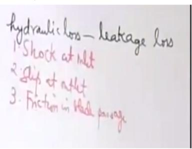
So these are basically hydraulic losses plus there also could be a leakage loss. So in terms of these losses we may determine the corresponding efficiencies. So if we say consider something called as hydraulic efficiency. So what is the hydraulic efficiency of a pump? So all the efficiencies consider certain losses, if there were no losses the corresponding efficiency would be 100%.
