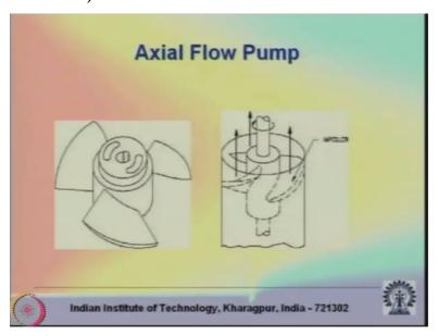
That means at the inlet the resultant flow is in the axial direction, this is like beta 1 the blade angle and this is alpha 1 which we have taken as 90 degree. Just try to draw an analogy
