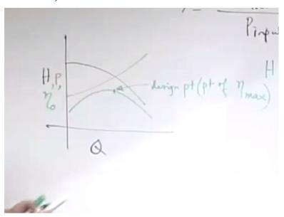
So it is drawn without considering that what are the piping and fittings and all those things which are there in the connecting system that connects from the sum to the supply reservoir. So the system has its own characteristics. What are the characteristic of the system? So if you see the system, so if you have a pump like this let us draw it schematically. Let us say that you have a pump that is having a supply to a reservoir.
