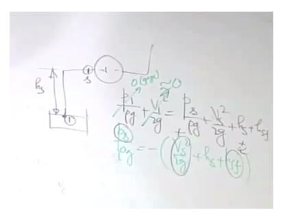
Now one has to keep in mind here that like no matter whatever is the Hs positive or negative, this is the location which is prone to very low pressure. So we have to put a lot of attention on this one and we can infer that if the pressure at this point is<the corresponding vapour pressure then you may have a cavitation. So we may consider that a safety margin. What is that? Ps/rho g-P vapour/rho g. We are talking about head so we are dividing it by rho g.
