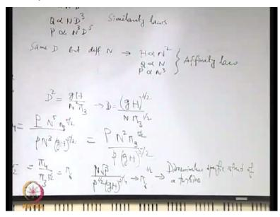
So you get N root P/rho to the power 1/2\*gH to the power 5/4, that is pi6 to the power 1/2. This is dimensionless specific speed of a turbine, okay. Now here also you can have equivalent dimensional form, what will be its equivalent dimensional form?
