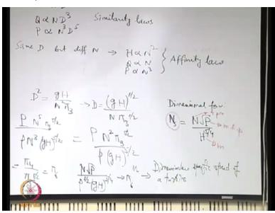
So if you have a dimensional form NS=N root P/H to the power of 5/4 because rho and V are non-variables that you are considering, right. So this is a dimensional form of a specific speed of a turbine and again the interpretation is very very similar as we had for a pump. The units again it depends on the country and the standard units for these which are used for the typical industries.
