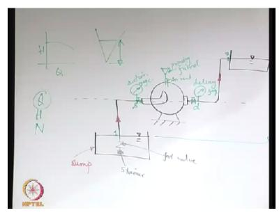
So if you have such a pump in a system, so let us just try to sketch it. Say you have, we are just drawing it very very schematically. So you are considering that there is a pump which is there in a system and so the direction of flow is, the pump is sucking the fluid from the supply and delivering it to the delivery and this is just a schematic way of representing the impeller because here our focus is how the pump behaves in a system and not so much on the details of the impeller.
