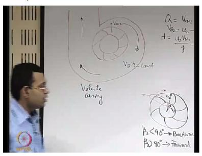
If you say have an impeller like this, then let us say that we are having a casing around the impeller. How is the casing? The casing is such that its area is continuously increasing. I am just magnifying it a bit too much but that will give you a sort of clarity in the nature of the casing. So the whole idea is that the fluid is leaving the impeller, entering the casing, coming like this and going out.
