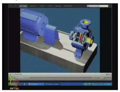
There is a motor which is inputting some electrical form of energy. So there is a shaft of the motor that is connected by a coupling to the shaft of the impeller, the name of the rotor is impeller, on which the rotor is there. So what is happening is, it is imparting some rotational form of energy to the impeller and the impeller therefore is rotating. Now a fluid will come and it will strike the blades of the impeller.
