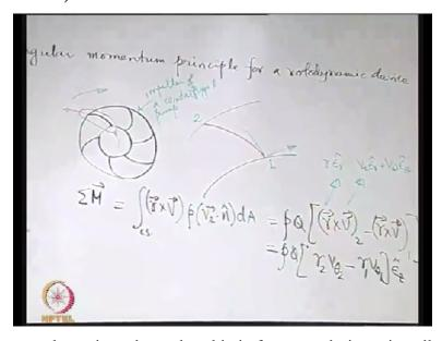
So let us just draw a schematic and say that this is for example is an impeller of a centrifugal pump. Just as an example. So now if you concentrate on these things, see these are like individual blades, okay. So these blades, what they do? So the fluid enters the blades and it leaves the passage which is adjacent to the blades. So the blades give a change in direction to the flow and because of the change in direction, you are basically having the change in angular momentum.
