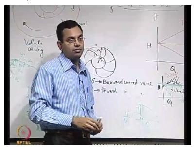
Even when you have Q=0, there is some H. So why you require this H? So this is some head that you need to develop to just overcome friction because before initiating the flow rate, you must have a threshold head or energy to overcome the frictional effects. So this is a threshold head or a threshold energy that needs to be available to overcome the friction and that is why it is not that at Q=0, H is 0 but some H to minimise or to overcome the frictional effects.
