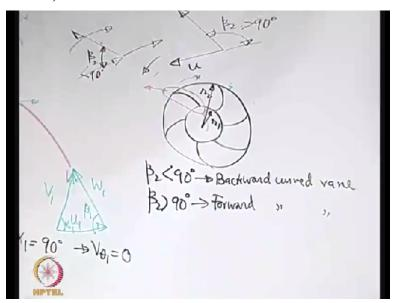
You have a direction of the relative velocity and you just make the angle between them. Let us say that the impeller is now moving in the opposite directions, that is it is instead of moving clockwise, it is moving anticlockwise. Then this is the direction of U, if it moving in the anticlockwise direction and then this is the velocity relative to the flow and you see that this angle, what is the convention?
