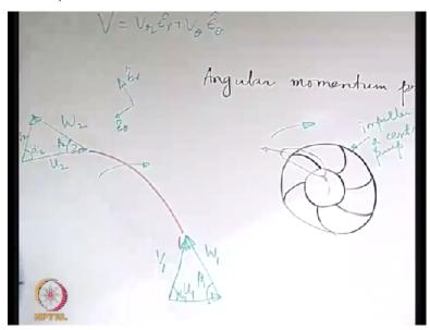
So first of all consider that when the fluid is entering the impeller, what it has? It has a velocity relative to the impeller. So let us say that this is the velocity that the fluid is having relative to the impeller. So these are the symbol that we will be using. Different books use different symbols but just we will be using some consistent symbols. So we will use W for velocity, relative velocity of the fluid, okay.
