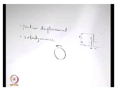
And based on that, one may have either a positive displacement type of fluid machine and the other type is a rotodynamic fluid machine. The positive displacement type of fluid machine, what it basically does? It relies on the change in volume of a fluid in a given confinement. We will give an example. Let us say that you have piston and a cylinder and say there is some compressible fluid which is being there, contained in the piston/cylinder arrangement.
