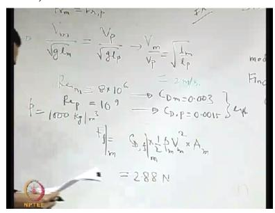
So what are the extra things. The Reynolds number of the model is 8\*10 to the power 6, the Reynolds number for the prototype is 10 to the power 9 and you can clearly see that these 2 Reynolds numbers are different because you cannot simultaneously satisfy these 2 that is what we have seen and from the experimental data of CD versus Reynolds number from this the CD for the model is 0.003.
