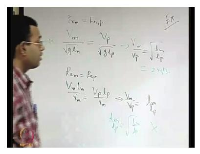
So if you consider that that similarity, then you have V model/square root of gl model=V prototype/square root of gl prototype. This is for that is considering the wave making resistance. So Froude number of the model same as Froude number of the prototype. Also if you consider the viscous resistances, then Reynolds number of the model and Reynolds number of the prototype, they should be identical.
