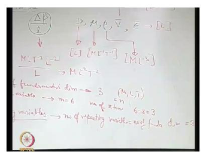
Example, let us say that you want to estimate the pressure drop in a pipe of a given length l. What is important for us is the pressure drop/length because we know that dpdx is physically what is the important parameter. It is a dependent parameter. It is a function of which variables? So if you have pipe of say diameter D in which a fluid is flowing, then what are the parameters on which we should depend.
