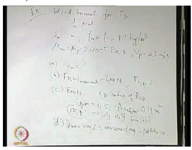
Let us say that we have one wind tunnel experiment. Wind tunnel for that force determination. The scale is 1/4th scale and it is a test on an automobile with the length of the model as 1 meter, the density of the model and density of the prototype, when we say density of the model and prototype, these are not densities of the solids actually. These are densities of the fluids flowing around.
