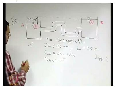
So we have a piping system like this. It is connecting 2 reservoirs of large extent. The values of
