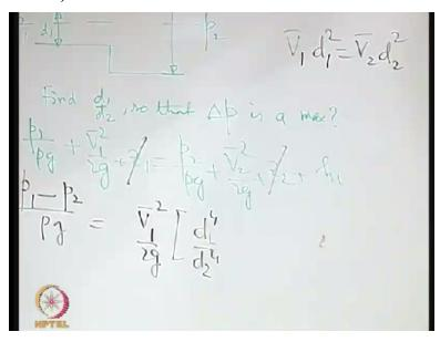
Then you can write say p1-p2/rho g=, now you can express V2 in terms of V1 by noting A1V1=A2V2, that means, you have V1\*d1 square=V2\*d2 square. So you can write V2 square/2g as V1 square/2g\*d24... sorry the other way. D1 to the power 4/d2 to the power 4.
