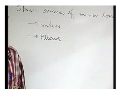
So other sources of minor losses are like presence of valves. So if there are valves in a pipeline. So what does a valve do?
