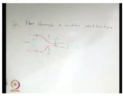
We will take another example, flow through a sudden contraction. So for flow through a sudden contraction, the idea is that the fluid is flowing from a pipe of a larger size to a pipe of a smaller size and when the fluid is flowing in that way, let us see that what happens to the streamlines. We have encountered such cases earlier and from our previous experience, we know that the streamlines first of all they will tend to get converged because the area is suddenly reducing.
