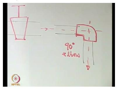
So if you have a pipeline say like this and you put a valve in the pipeline. We are not drawing a valve in a proper detailed manner but just let us say this is a schematic way of representing. So let us say that this is a physical obstruction. So when this is lifted, the entire fluid may flow. When this is put down, depending on the extent to which it is put down, it will restrict the motion of the flow or motion of the fluid.
