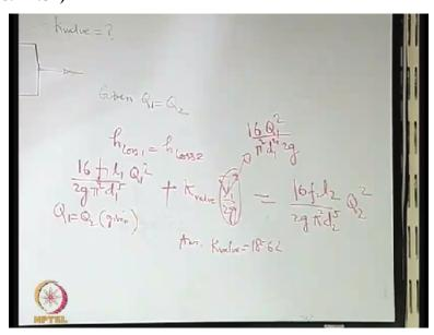
So h loss 1=h loss 2. So what is h loss 1? You have f111/d1, or we write in term of Q. 16f111Q1 square/2g pi square d1 to the power 5+the k valve \*V square/2g, so V1 square/2g is as good as, V1 is 4Q/pi d square. So 16Q1 square/pi square d1 to the power 4 2g, that is V1 square/2g=the head loss at 2, that is 16f212/2g pi square d2 to the power 5\*Q2 square, right and it is given that Q1=Q2, given.
