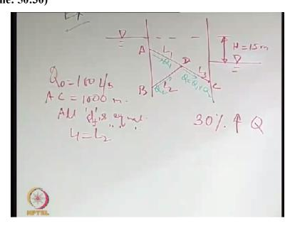
The problem statement is like that initially, so you can see that here there are pipes AD BD and DC. So this is just shown by schematic, so not the with being shown. So here initially only the part AC was there. There was no branch BD and then the flow rate was 100 liter per second that is given. So Q0 is 100 litre per second and the length of AC is 1000 meter that is 1 kilometer. To increase the flow rate, another pipe BD is added, okay.
