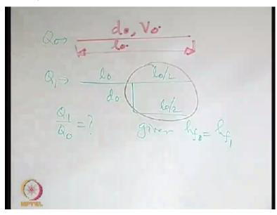
It has a diameter say d0 and the velocity V0. It is having some length say 10. To increase the flow rate, a new arrangement is made. What is the new arrangement? The new arrangement is a branch is taken away from the midpoint of this one. So this is 10. This is 10/2 and this 10/2. So the diameter is the same. The diameter is d0 for the second arrangement as well.
