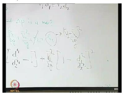
and then you have -1 for 1 V1 square/2g, then what is this head loss? This is just V1-V2 whole square/2g, this is sudden expansion loss. The lengths are not substantial to have major losses as important. So here this is an example where we will see that minor loss is the dominating one. So the length is so short that the loss due to the length is not. Of course it is there but that may be neglected as compared to this loss.
