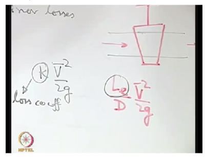
So for all these, it is not so easy to calculate or rather write analytically exactly the expression for the loss but one may have whole amount of experimental or computationally available data and from that, the loss is somehow characterised as k\*V square/2g. The idea is straightforward that you are trying to write the loss as in proportion to the kinetic energy rate and the motivation is
