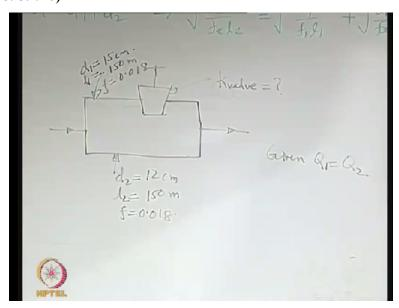
So you have 2 pipes, 2 pipelines and these 2 pipes, the upper one is d1=15 centimeter and length is 150 meter, the friction factor is a constant which is 0.018. The other pipe is, the diameter d2 is
