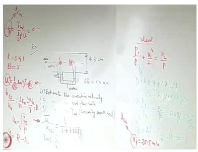
Let us say that you have a piping system or a single pipe in this example, where a pitot tube is put, the fluid that is being handled in the system is air, and the manometric fluid is water, the difference in the height of the 2 limbs of the manometer say is delta h which is given, the diameter of the pipe is 8 centimeter and the pressure upstream is one atmosphere approximately 101 kilopascal.
