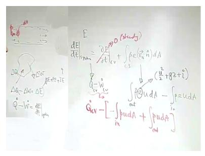
The objective will be to figure out that how the head losses are related to the total energy balance, let us say that you have a pipe of whatever sections, say a circular pipe as an example and we are looking for the fluid in the pipe, and trying to write an expression for the energy balance. So for any conservation equation we may start with the Reynolds transport theorem, so let us start with the Reynolds transport theorem, where E is the total energy of the system.
