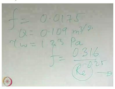
So for a smooth wall, it will depend on only the Reynolds number, and for the hydraulically smooth pipe this is like 0.316/Reynolds number to the power 0.25, otherwise one may directly read from the Moody's diagram the corresponding graphically plotted values without looking into the function. So that means if you know f, you will get a Reynolds number right, and the Reynolds number is what?
