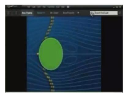
Let us see it as a simulated example. So if you see 2 Eddies of counter rotating nature are formed at the back or in the low pressure region or in the wake side of the cylinder. We are talking about still low Reynolds number cases.
