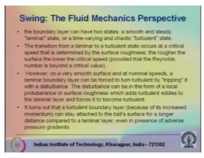
So now the question is that like as we first were discussing that what should be the effect of the speed of the ball say the speed of the ball is 145 kilometer per hour and say it is a new ball, it is equally turbulent in all sides, so the resultant side force is 0 so to say. That means if you have a very fast bowler and is holding a straight sort of seam or maybe is not holding a straight seam but with an inclined seam.
