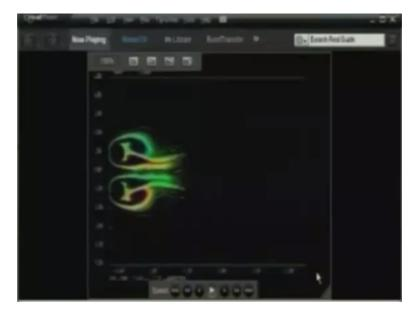
So you may have even multiple cylinders and with multiple cylinders these types of effects you can see with like as if one effect is getting superimposed on the other. Here the symmetry sort of is very well preserved because the Reynolds number is not that large but the symmetry may be destroyed by advection of vorticity if the Reynolds number is substantially larger. **(Refer Slide Time: 27:57)**
