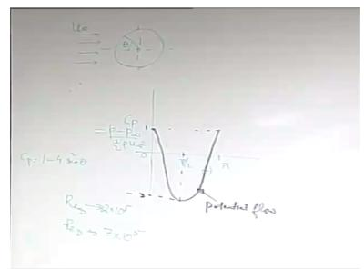
So if you want to plot the pressure distribution around the cylinder, so when we plot a pressure distribution we basically plot the Cp versus theta so Cp is the pressure coefficient p- p infinity/1/2 rho u infinity square. So the physical situation that we are considering is there is the circular cylinder and there is a flow past this circular cylinder. Flow is coming with the velocity of u infinity.
