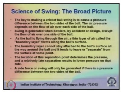
So we will try to see that how these swing balls are going to be affected in terms of a scientific perspective, so the science of swing the broad picture. So as we have discussed earlier that the key to have a cricket ball swing is to cause a pressure difference between the 2 sides of the ball. It is not just true for a cricket ball; it is true for any other ball that we may look for.
