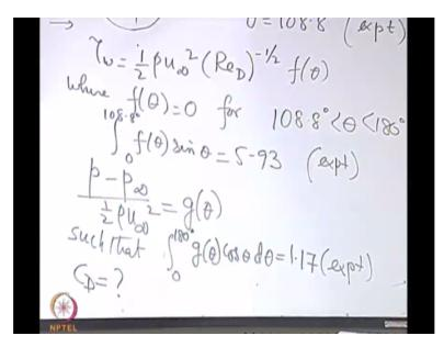
Let us say that, you have a circular cylinder with p infinity, u infinity as the free stream conditions, measure an angle theta from this direction. And it is given that boundary layer separation occurs. We will see that when boundary layer separation occurs in such a case in detail later on. But, say for this problem, it is given that boundary layer separation occurs at theta=108.8 degree, this is from experiments.
