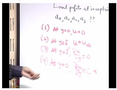
Let us say that, we want to have an estimation of the velocity profile at the point of separation and let us say that it is given in this form u/u infinity=a0+a1y/delta+a2. This is an example of assume that this is velocity profile at the inception of separation. Our objective is to find out a0, a1, a2, a3 consistent with the physical conditions. So, it is just like estimating a velocity profile or fitting a velocity profile in a polynomial form that we did for flow over a flat plate.
