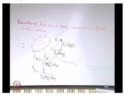
So, the resultant force on a body immersed in a fluid under motion. So, do not confuse it with fluid statics. It is not fluid at rest. So, we are not talking about forces like buoyancy forces like that. So, this is solely because of the relative motion between the fluid and the solid. Whatever is the force that force we want to identify. So, generally the convention is that, let us say you have an arbitrary shape body.
