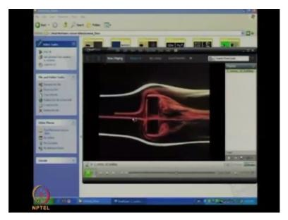
This is flow past a building. So, it is basically a building simulated and if you see that there is a flow separation and there is low pressure region in the back. So, whatever is the region which is towards the right after the boundary layer separation has occurred that is a low pressure region. And it strongly depends on the shape. So, let us look into the case if you change the shape, what happens?
