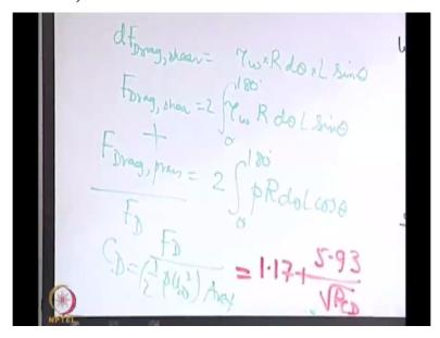
So, that is tau all\*Rd theta\*the length of the cylinder. That is number one but, what you want is the drag force, coefficient of drag so, you want the force component of this in the direction of the flow. So, what will be that? So, basically this\*sin theta. So, you will have dF drag due to shear=tau all\*Rd theta\*L\*sin theta okay. So, you have the total drag force due to shear=tau all\*Rd theta L sin theta integrate 2\*0 to 180 degree right.
