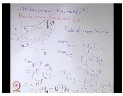
So, let us write what is the momentum flux or may be rate of momentum transfer. So, the rate of momentum transfers at A, what is this? So, what is the rate of mass transfer at A? rho u infinity\*delta, that multiplied by u infinity is the rate of momentum transfer at A. what is the rate of momentum transfer at B? again one part within the boundary layer, another part outside the boundary layer.
