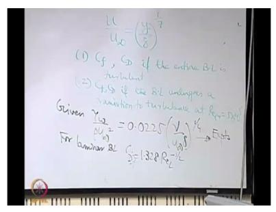
Sometimes, one also uses a third parameter which is known as the shape factor H, which is given by delta star/theta. The ratio of these 2. Why it is given a name of a shape factor is somewhat obvious. The obvious is that, this ratio depends solely on the shape of the velocity profile. Because, if you see the integrals, this integrals of course they themselves depend on the shape of the velocity profile but sort of even their ratio also therefore depends only on the shape of the velocity profile.
