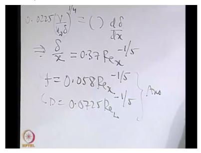
So, let us first write tau all/rho u infinity square=ddx of integral 0 to delta u/u infinity\*1-u/u infinity dy. So, this part you may substitute u/u infinity as a function of y/delta and then you will get this as something\*d delta dx that is fine. Substitute u/u infinity as y/delta to all these. Now, what about tau all? See, if you want to calculate mu du dy at the wall, you see that, that you cannot calculate using this velocity profile.
