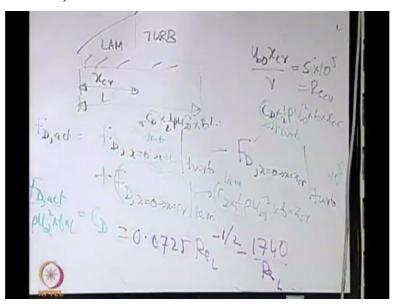
So, you may have the flat plate in this way. You have first a laminar boundary layer, then it undergoes a transition to turbulent boundary layer. Let us say that this is the length x critical over which it is laminar and then beyond that, it is turbulent. So, the question will be that, what is the length of your plate? If the length is > x critical, how do you find out x critical? X critical is given by u infinity x critical/mu is 5\*10 to the power 5, that is Re critical.
