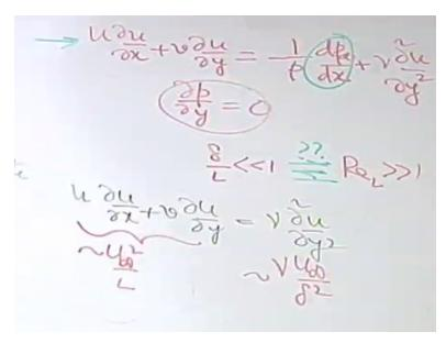
But here you have u infinity gradient is 0, u infinity is constant for flow over a flat plate, so du infinity/dx=0 which implies the dp infinity/dx=0. So for flow over a flat plate the dp/dx is 0, so when you have dp/dx=0, then you are left with your momentum equation with this one okay. So if you write the order of magnitude of the different terms here, the left hand side order of magnitude is u infinity square/L, and the right hand side is nu u infinity/delta square right.
