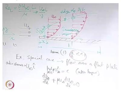
So let us take an example of flow over flat plate, special case flow over a flat plate. First of all, what is our objective is to find out what is this dp infinity/dx okay, let us consider the outer stream. See the outer stream the free stream flow is u infinity, so the velocity field is like u infinity i in the outer stream, the outer stream u is u infinity i, you can clearly understand that this is an irrotational flow, because no gradient in the velocity.
