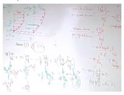
Keeping that in mind let us write the ratio of the inertia terms and the pressure gradient term order of magnitude, this is of the order of inertia term is of the order of u infinity square delta/L square, and pressure gradient term of the order of u infinity square/delta. So this becomes of the order of delta/L whole square right. Therefore, if delta is <<1 see so many simplifications are possible just by this consideration, so this becomes one of the very key considerations.
