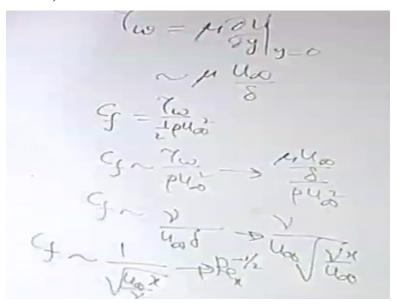
So what is the wall shear stress? The wall shear stress is the mu\*del u/del y at the wall y=0, so what is the scale of the wall shear stress? What is the order of magnitude of this? mu\*u infinity/delta right. So important non-dimensionalization of wall shear stress is what? We have seen it earlier in an example when we are dealing with Navier Stokes equation that is the friction coefficient Cf=tau wall/1/2 rho u infinity square.
