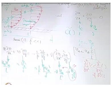
That you have a flat plate, the plate is confronting a free stream of fluid with a velocity of say u infinity, now when this fluid is coming in contact with the plate, what is happening that is what we are interested to see. Clearly, when we consider say one section, and we go further and further away from the plate, the physical phenomena tend to get changed. How it tends to get changed?
