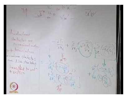
So when we discussed about homogenous turbulence, this terminology at least we introduced in the previous lecture and what we remarked is that, if you have a homogeneous turbulence, it means that the turbulence statistics are independent of position. So that means if you have say u1 prime square at a point, then if you go at different points, you will get the same turbulence statistic.
