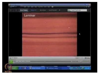
So in these experiments, some coloured dye was there and you see that it is a layer by layer motion of fluid elements. Say this is also a tube, flow-through a tube experiment. So it is a laminar flow. So there was a coloured dye that was injected and the coloured dye is just following a parallel sort of motion.
