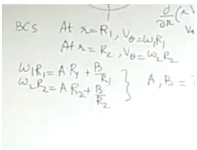
So the boundary conditions are at r=R1, v theta is omega 1\*R1 no-slip boundary condition so velocity of the fluid same as velocity of the solid and at r=R2, v theta is omega 2\*R2. So you substitute that so omega 1 R1=Ar1+B/r1 and omega 2 R2=Ar2+B/r2 so it is possible to find out A and B from these two right. These are like capital as per our notations, so AR1+B/R1 AR2+B/R2.
