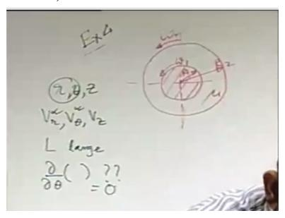
So you have 2 concentric cylinders of radii R1 and R2. Let us say that the inner cylinder is rotating with an angular velocity omega 1 and the outer cylinder is rotating with an angular velocity omega 2 and these angular velocities are like these are not functions of anything, these are constant angular velocity then we are considering a steady flow of a Newtonian fluid of constant properties in which the fluid is kept in the gap between the 2 cylinders.
