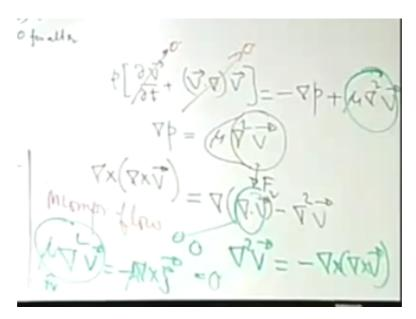
So the momentum equation is rho okay. So this is the vector form, we have derived this vector form and the advantage with the vector form is whatever vector operation that we will be doing on it so longer as it is in a vector operation form we do not explicitly mention which coordinate system it is, so it remains valid for all types of coordinate systems.
