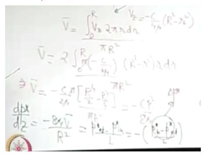
So this we just write as p star out-p star in/L. So in other words it is – of p star in-p star out/L. I mean why we are writing it in this way is see the p star in-p star out is the driving delta p star for the flow, the driving difference in piezometric pressure that should drive the flow. See why this driving pressure difference is necessary? It is necessary because you have viscous resistance in the flow.
