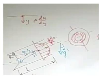
So if you have a solid boundary like this, if you have this as y then you have like mu du/dy. So y is away from the solid boundary towards the fluid. The reason is you want to write it as a positive shear stress, so you want u to be increasing in the y direction. So y=0 is like the noslip and then u increases but here the r direction is opposite to that so you have to make it up with the –sign.
