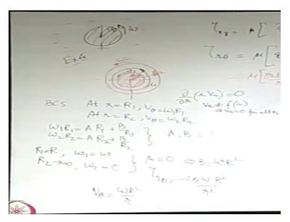
So the modified problem is you have one single cylinder, solid cylinder rotating with an angular velocity omega in a fluid of large extent. So one cylinder of radius r and of large length rotating with omega, so there is no inner or outer concept. So how can you solve this problem by considering the solution of this one? So omega 1 so R1=capital R, omega 1=omega, R2 tends to infinity and omega 2=0.
