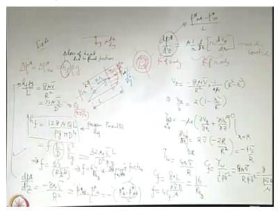
So the viscous resistance therefore you may say that delta p star is nothing but the delta p star because of the viscous resistance and we may write it in terms of a head or some unit of length so we remember that the pressure is nothing but some length unit\*rho\*g and the length unit is the equivalent unit of pressure expressed in terms of length with which we call as head so that is what we discussed also earlier.
