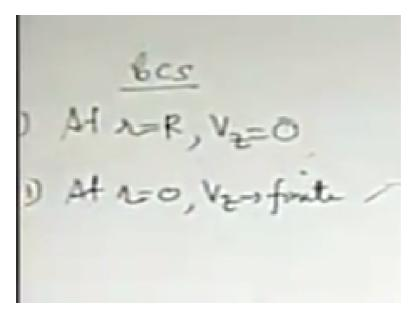
Boundary conditions, so one of the boundary conditions that is at the wall is straightforward at small r= capital R you have vz=0 no-slip boundary condition. Then what happens at small r=0 that is a point of singularity so to say but physical problem is that vz has to be defined at small r=0 I mean you cannot have a situation where there is vz undefined at small r=0 because it is a physical problem the pipe is entirely filled up with fluid with some velocity.
