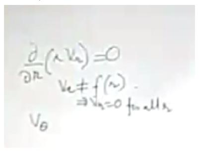
No gradient with respect to z, so that term is 0. So only one term is R\*vr the derivative of that that means d/dr of rvr that is=0, just like what we had for Hagen-Poiseuille flow and what will be the obvious conclusion that vr is not r\*vr or vr is not a function of r. So we know that at 2 different radii vr is 0, R=R1 and R=R2 and that is good enough for us to say that vr=0 for all r because vr is not a function of r.
