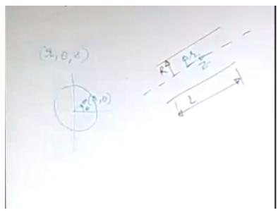
So you have a pipe of say maybe we are talking about an axial length of L and fully developed flow. So the coordinate systems what we use for this case are the cylindrical polar coordinate systems, which are more common. So you have small r as the radial coordinate, z as the axial coordinate and if you take the cross section of this, so if you draw separately the sectional view, it is a circle.
